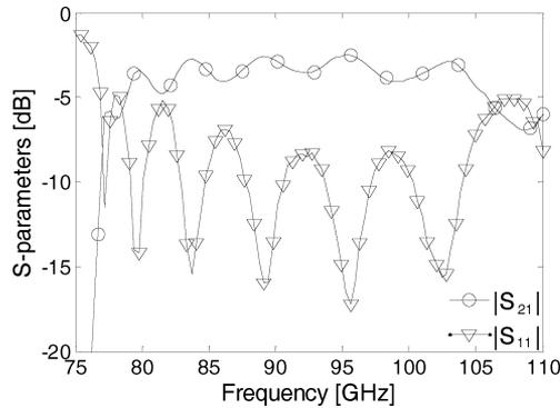
Fig. 4. S-parameters of 2.5 mm waveguide with transitions.
