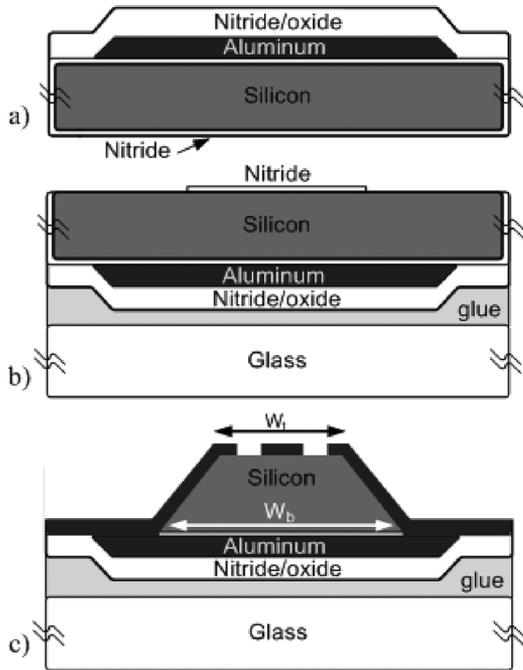
Fig. 1. Technology steps. After aluminum deposition (a), the silicon wafer is glued top down to a glass carrier (b), and waveguide sidewalls are defined via KOH etching (c).
