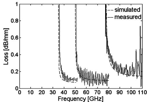
Fig. 6. Waveguide losses: simulations versus measurements comparison. Losses are expressed as  $10 \cdot \log_{10} \exp(-2 \cdot \alpha \cdot d)$  choosing  $d = 1$  mm.
