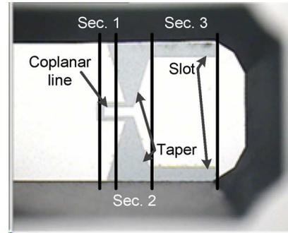
Fig. 3. Optical microscope photo of coplanar-to-waveguide transition. Waveguide sidewalls are in black (off-focus), and the top metallization in white, on which the slot transition can be seen in light grey.
