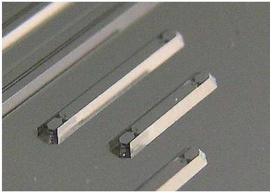
Fig. 2. Waveguides camera made picture. Metal layers are in dark grey, sidewalls in light grey, and transition slots in black.
