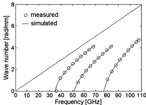
Fig. 5. Dispersion diagram: simulations versus measurements comparison. The straight line corresponds to the case of a TEM mode in silicon.
