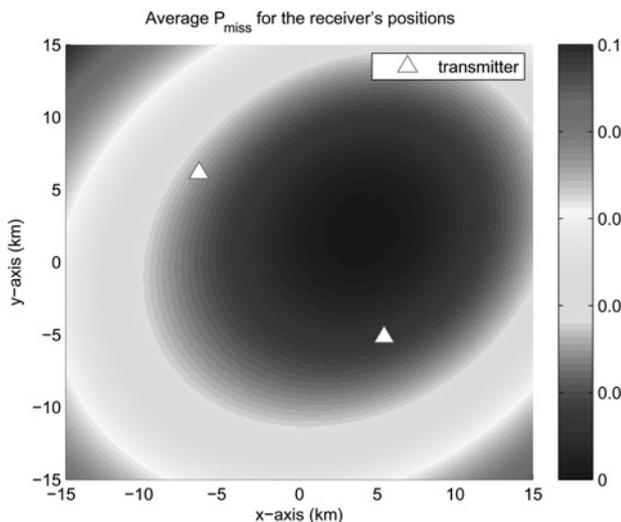
Fig. 5 Average  $P_M$  (weighted by the priority function) obtained by changing the receiver's position
