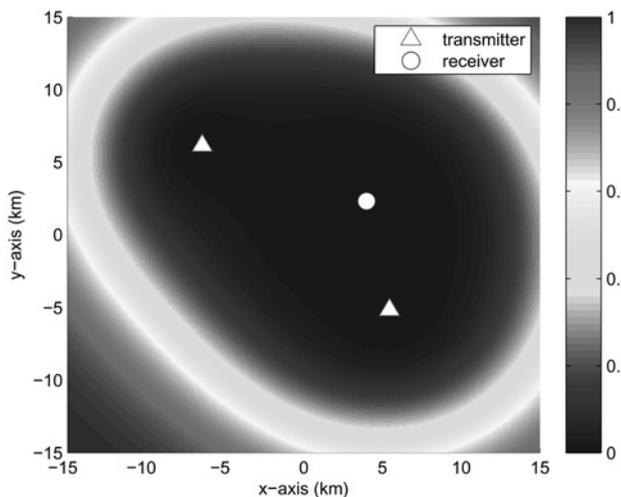
Fig. 6  $P_M$  obtained for different target positions after placing the first receiver
