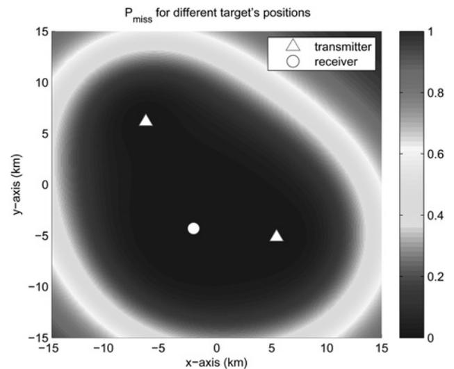
Fig. 3  $P_M$  for different target's positions
