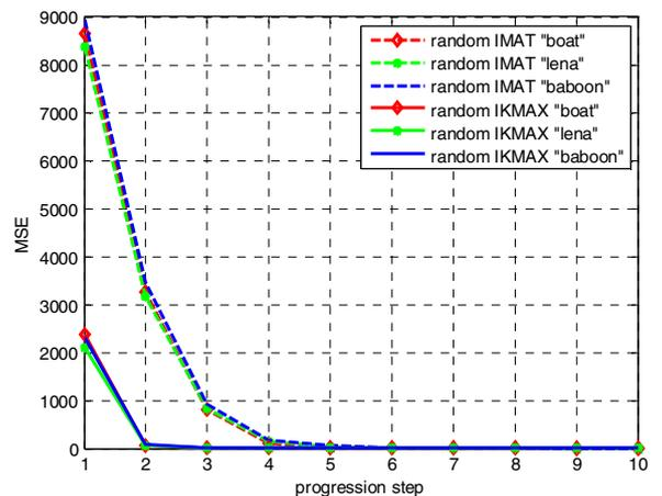
Figure 4. The MSE of the proposed method versus the progression step for random sampling.
