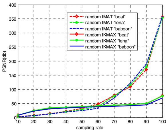
Figure 6. The rate distortion performance of the proposed method for random sampling.
