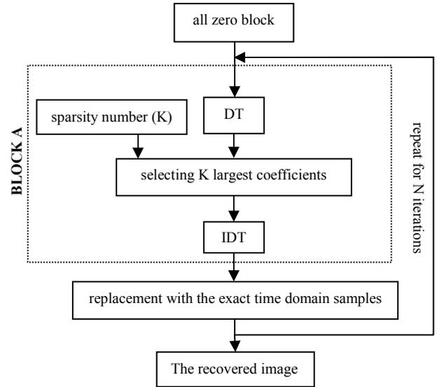
Figure 2. Block diagram of IHT.
