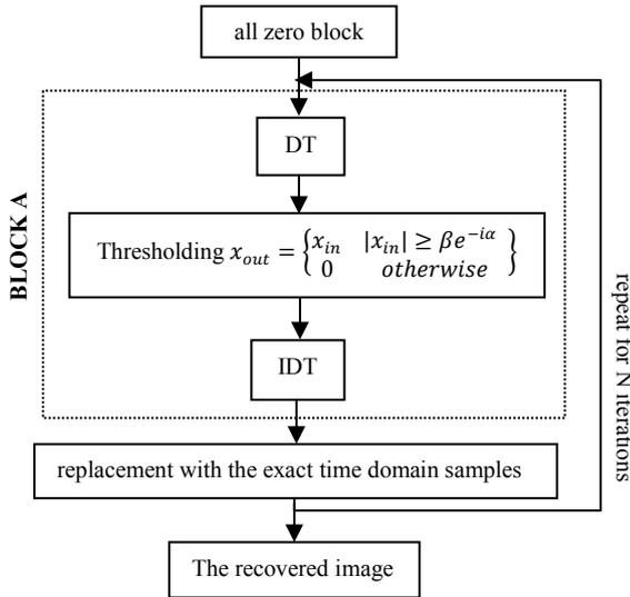
Figure 1. Block diagram of IMAT.
