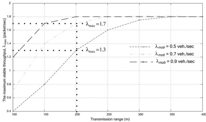
Fig. 6 Maximum stable throughput against TR
