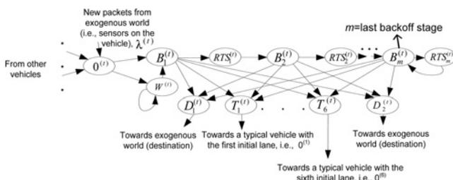
Fig. 4 QN model corresponding to a typical class- $t$  vehicle
