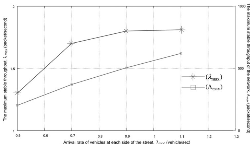
**Fig. 5** Maximum stable throughput against arrival rate of vehicles
