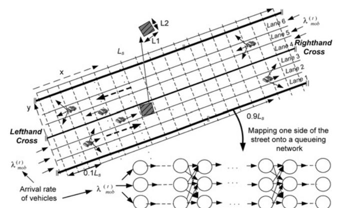
Fig. 2 Mobility patterns of vehicles in a typical street
