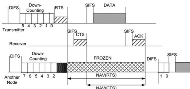
Fig. 1 Packet transmission in IEEE 802.11
