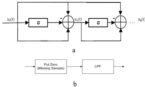
**Fig. 1. a)** The reconstruction block diagram using standard iterative method and **b)** The block  $G$  in the standard iterative method
