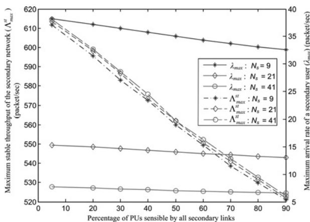
**Fig. 5** Effect of spatial distribution of PUs on the maximum stable throughput of the secondary network
