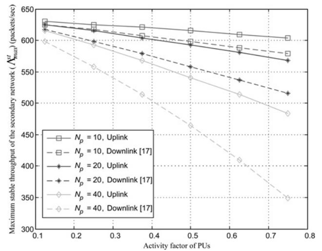
**Fig. 6** Effect of activity factor on the maximum stable throughput of the secondary network
