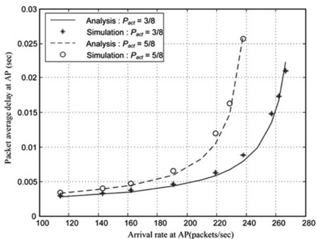
**Fig. 8** Analytical and simulation results for average delay corresponding to the packet transmissions by AP
