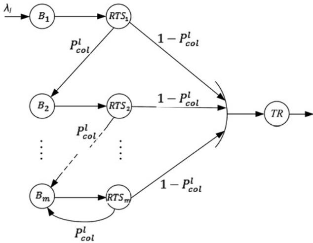
Fig. 2 Proposed queuing network to model a typical SU
