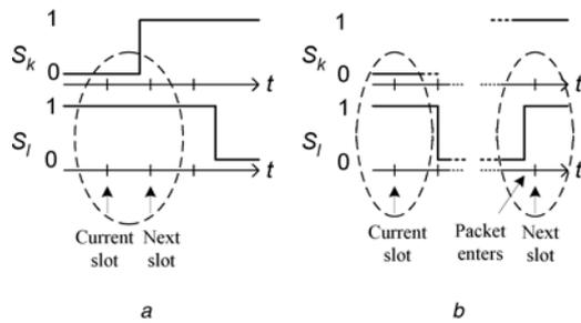
**Fig. 4** Diagrams depicting the status of next slot relative to current slot
