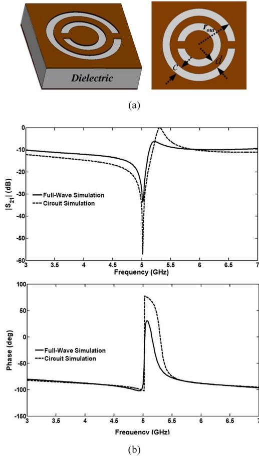
Fig. 3. (a) Geometry of the unit cell of CSRR loaded dielectric parallel-plate waveguide. (b) Transmission and phase characteristics for the unit cell of CSRR loaded dielectric parallel-plate waveguide. The dielectric has thickness  $h = 0.5$  mm and dielectric constant  $\epsilon_r = 15.3$ . CSRR dimensions are  $r_{out} = 1.5$  mm and  $d = c = 0.3$  mm. Extracted parameters of equivalent circuit are  $C_c = 0.54$  pF,  $C = 1.54$  pF,  $L_c = 0.48$  nH.
