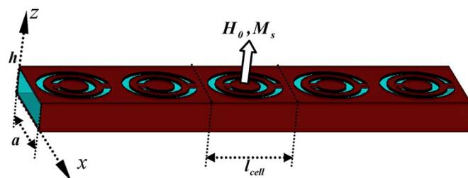
Fig. 1. Geometry of the proposed transversely magnetized ferrite rectangular waveguide periodically loaded with CSRRs. The number of cells  $N = 5$ .
