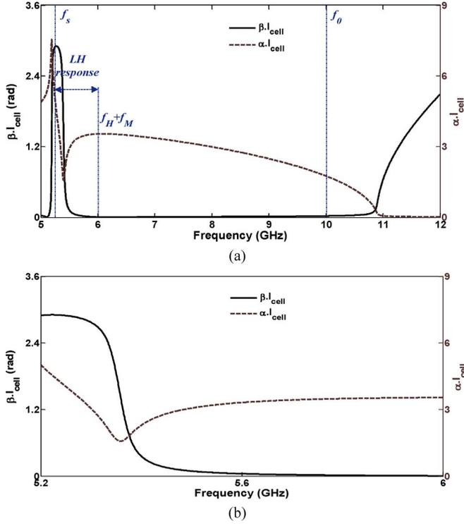
Fig. 5. Dispersion diagram calculated by (6). (a) Frequency range from 5 to 12 GHz. (b) Magnification of the LH range from 5.20 to 6 GHz.  $h = 0.5$  mm,  $a = 4$  mm,  $l_{\text{cell}} = 4.5$  mm,  $H_0 = 400$  Oe,  $M_s = 0.173$  T,  $\epsilon = 15.3$ ,  $\alpha = 0.007$ ,  $C_c = 1.54$  pF,  $C = 0.54$  pF,  $L_c = 2(\mu)^{1/2}/(1 + (\mu)^{1/2}) \times 0.48$  nH.
