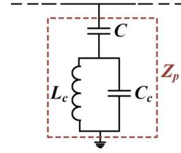
Fig. 2. Equivalent circuit model for the basic cell of the CSRR loaded transmission line.
