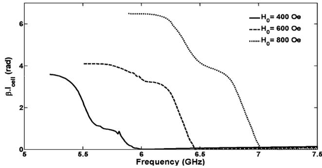
Fig. 7. Simulated phase shift per unit cell for the proposed LH structure under different magnetic bias fields.
