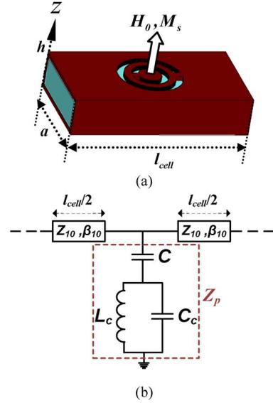
Fig. 4. (a) Ferrite rectangular waveguide loaded with the unit cell of CSRR. (b) Equivalent circuit model of ferrite rectangular waveguide loaded with the unit cell of CSRR.
