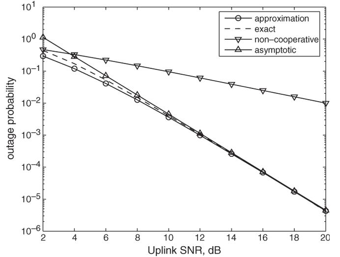
Fig. 4. Outage probability versus uplink SNR, where  $N = 128$ , target rate  $R = 1$ , and the Gaussian links are 6 dB stronger than the Rayleigh uplinks ( $\varepsilon = 4\varepsilon'$ ).
