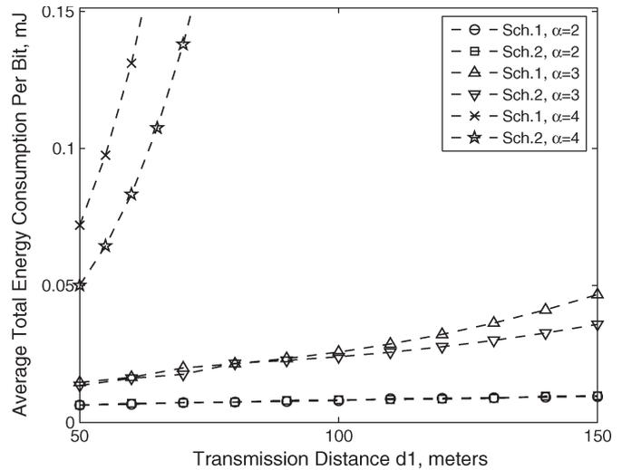
Fig. 10. Average energy consumption of the cooperative schemes one and two per bit versus the source distance from the gateway. We have used the parameters' values given in Table I.
