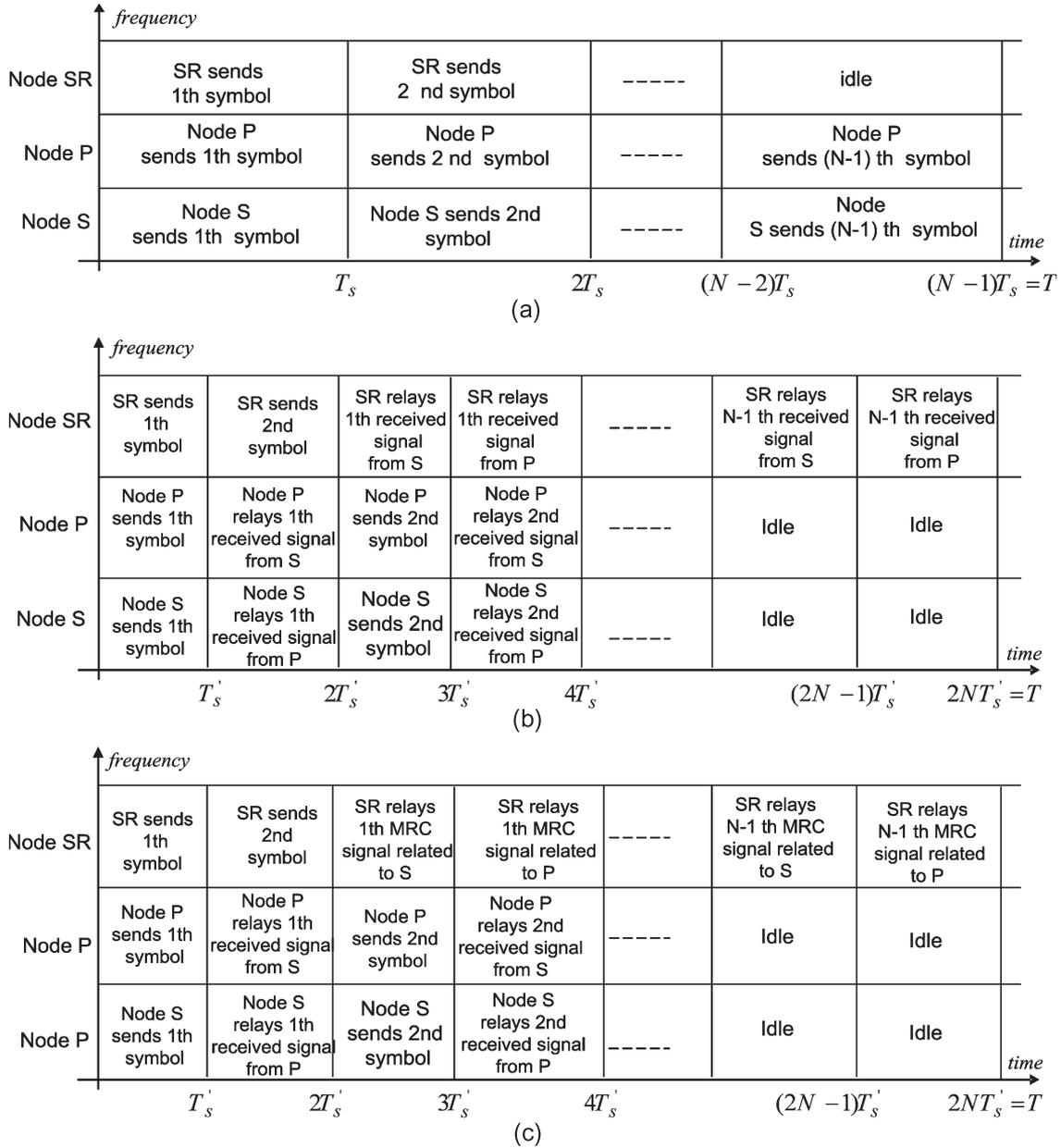
Fig. 3. Orthogonal channel assignment. (a) Noncooperative scheme. (b) Scheme one. (c) Scheme two.
