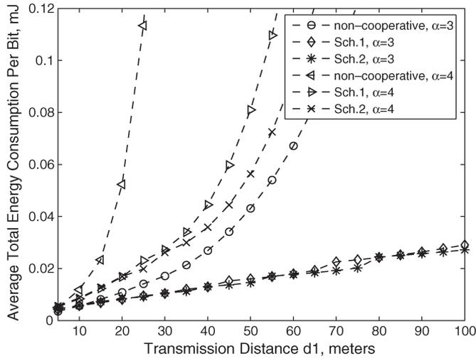
Fig. 9. Average total energy consumption per bit versus the source distance from the gateway. The path loss exponent is equal to 3 and 4.
