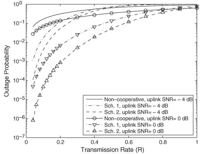
Fig. 7. Outage probability versus transmission rate  $R$ , where  $N = 128$ , and the Gaussian links are 6 dB stronger than the Rayleigh uplinks ( $\epsilon = 4\epsilon'$ ).
