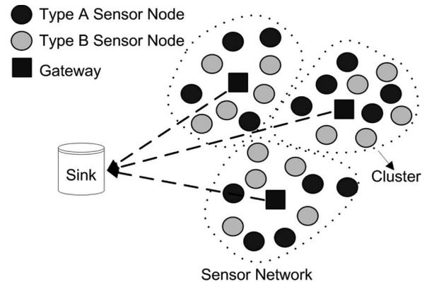
Fig. 1. Heterogeneous wireless sensor network with three types of sensor nodes.
