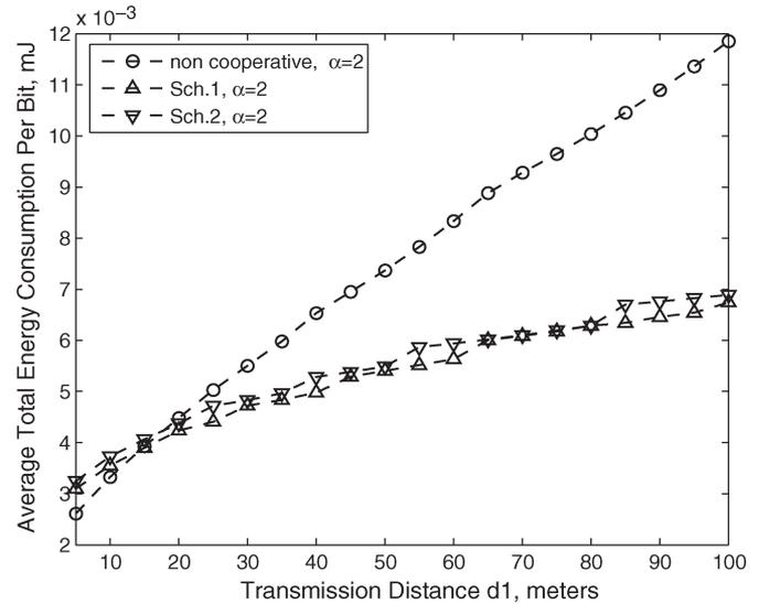
Fig. 8. Average total energy consumption per bit versus the source distance from the gateway. The path loss exponent is equal to 2.
