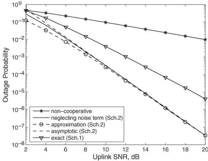
Fig. 6. Outage probability versus uplink SNR, where  $N = 128$ , target rate  $R = 1$ , and the Gaussian links are 6 dB stronger than the Rayleigh uplinks ( $\epsilon = 4\epsilon'$ ).
