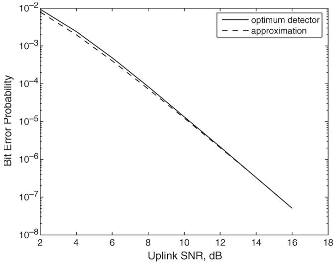
Fig. 5. Bit error probability versus uplink SNR. Gaussian links are 6 dB stronger than Rayleigh uplinks ( $\epsilon = 4\epsilon'$ ).
