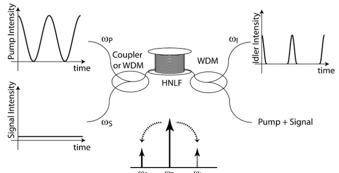
Fig. 1. Schematic of short pulse generation principle using single-pump OPA. WDM: wavelength demultiplexer/multiplexer; HNLF: highly nonlinear fiber.
