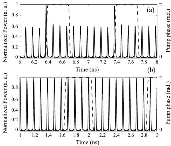
Fig. 6. (a) Train of generated pulses (solid line, left axis) and pump phase (dashed line, right axis) for a 3 Gb/s PRBS phase modulation. (b) Train of generated pulses (solid line, left axis) and pump phase (dashed line, right axis) for a 2.5 Gb/s PRBS phase modulation with an adjusted delay time.
