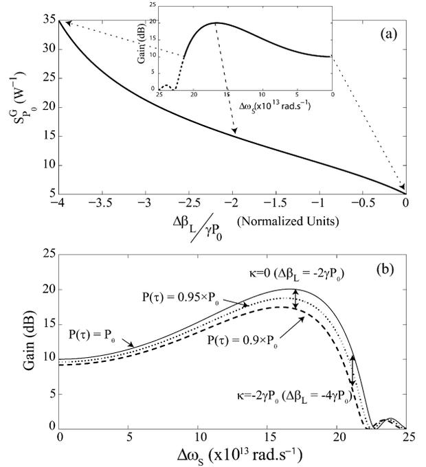
Fig. 2. (a) Sensitivity as a function of  $\Delta\beta_L$  normalized by  $\gamma P_0$ . The inset represents the corresponding gain spectrum for a typical HNLFF with dispersion parameters  $\beta_2 = 2.9 \times 10^{-29} \text{ s}^2 \cdot \text{m}^{-1}$  and  $\beta_4 = -6.4 \times 10^{-55} \text{ s}^4 \cdot \text{m}^{-1}$ . (b) Parametric gain spectrum for different pump powers.
