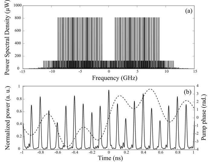
Fig. 5. (a) Spectrum of multitone phase modulated sinusoidal pump. (b) Train of generated pulses at the idler location (solid line, left axis) showing how it fluctuates because of pump phase fluctuations in time (dashed line, right axis).
