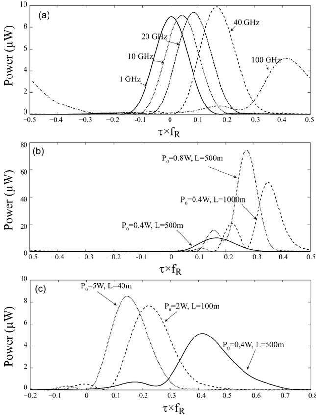
Fig. 4. (a) Generated pulse shapes for different repetition rates  $f_R$ . In all cases, we have  $\gamma P_0 L = 3$ . (b) Generated pulse at  $f_R = 20$  GHz for  $\gamma P_0 L = 3$  (solid line) and for  $\gamma P_0 L = 6$  with a doubled pump power (dotted line) or a doubled HNLF length (dashed line). (c) Generated pulse at  $f_R = 100$  GHz for different sets of  $P_0$  and  $L$  leading to  $\gamma P_0 L = 3$ .
