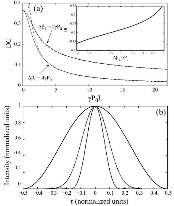
Fig. 3. (a) Duty cycle as a function of  $\gamma P_0 L$  for  $\Delta\beta_L = -4\gamma P_0$  and  $\Delta\beta_L = -2\gamma P_0$ , using the derived analytical expressions of (7) and (9) (solid line), and using the gain expression of (2) (dashed line). (b) Normalized temporal traces of pump (solid line) and generated idler for  $\Delta\beta_L = -2\gamma P_0$  (dotted line) and  $\Delta\beta_L = -4\gamma P_0$  (dashed-dotted line).
