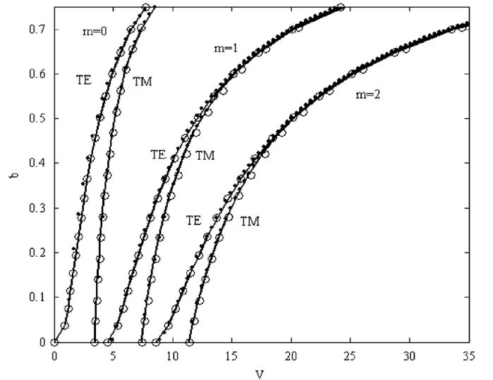
Fig. 8. Dispersion curves of waveguide with exponential index profile for TE and TM polarizations with  $n_0 = 2.5$ , and  $n_s = 3.8$ . Solid line: transfer matrix; circles: the proposed method; dots: polynomial expansion approach.
