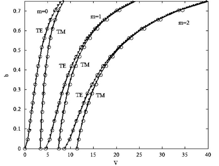
Fig. 7. Dispersion curves of waveguide with exponential index profile for TE and TM polarizations with  $n_0 = 2.177$  and  $n_s = 2.220$ . Solid line: transfer matrix; circles: the proposed method; dots: polynomial expansion approach.
