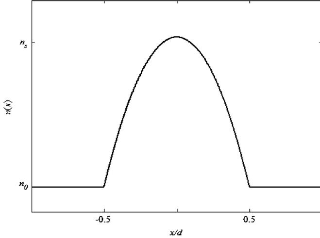
Fig. 6. Parabolic index profile plotted versus normalized distance.
