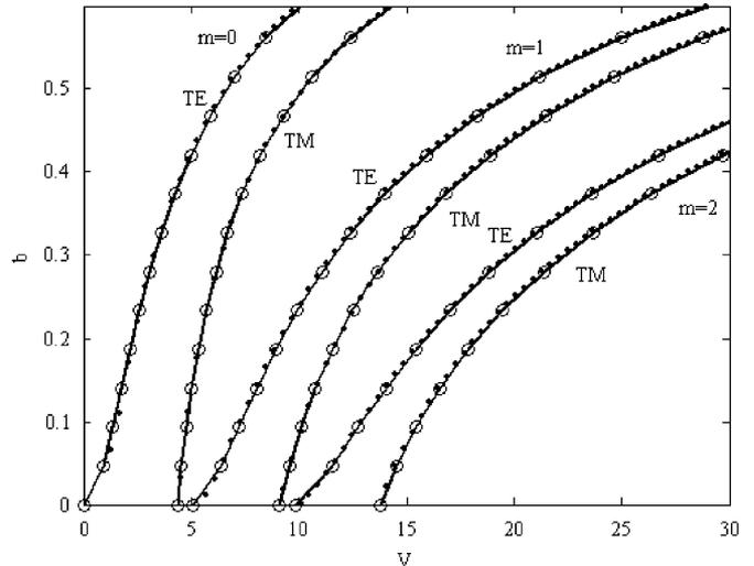
Fig. 4. Dispersion curves of a waveguide with exponential index profile for TE and TM polarizations with  $n_0 = 2.177$ , and  $n_s = 2.220$ . Solid line: exact solution; Circles: the proposed method; Dots: polynomial expansion approach.
