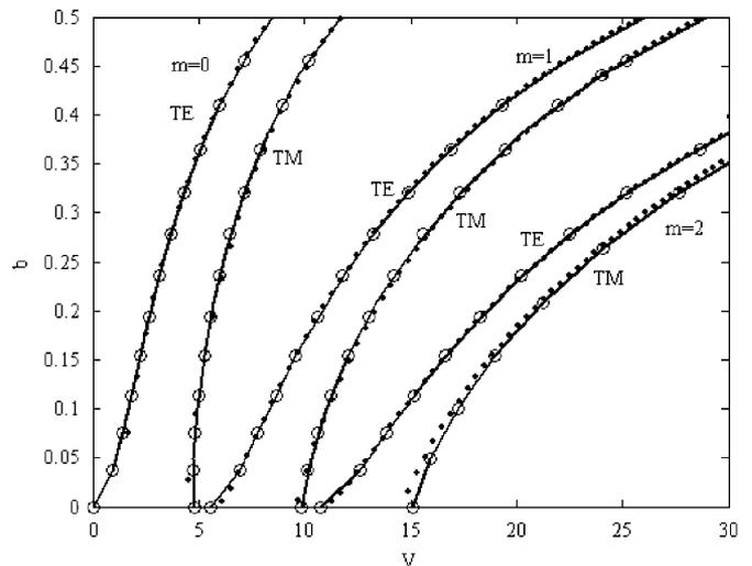
Fig. 5. Dispersion curves of waveguide with exponential index profile for TE and TM polarizations with  $n_0 = 2.5$  and  $n_s = 3.8$ . Solid line: exact solution; circles: the proposed method; dots: polynomial expansion approach.
