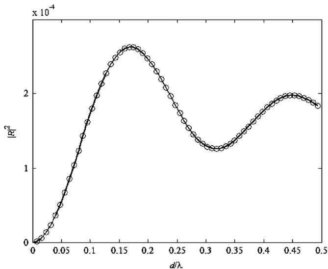
Fig. 3. Reflection coefficient of the structure shown in Fig. 2 with  $n_0 = 2.177$ ,  $n_s = 2.220$ , and  $\theta = 30^\circ$  for TE polarization. The solid line represents the exact results and the circles stand for the proposed method.
