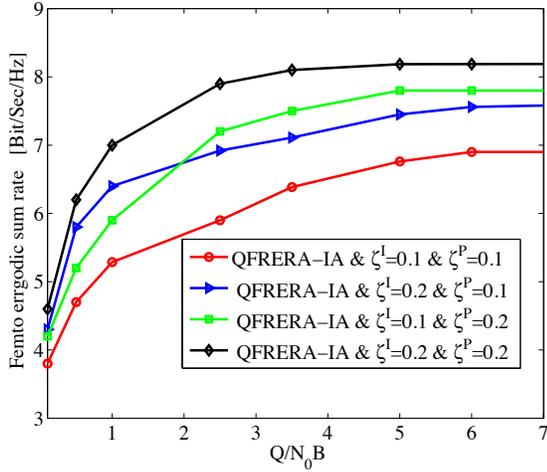
Fig. 3. Femto ergodic sum rate vs.  $\frac{Q}{N_0B}$  for QFRERA with different values of  $\zeta^I$  and  $\zeta^P$ .
