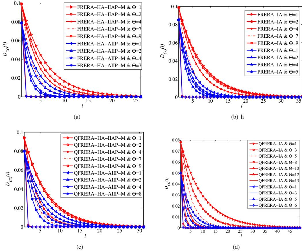
Fig. 5. The effect of the value of  $\Theta$  on the convergence speed of hybrid and iterative algorithms.
