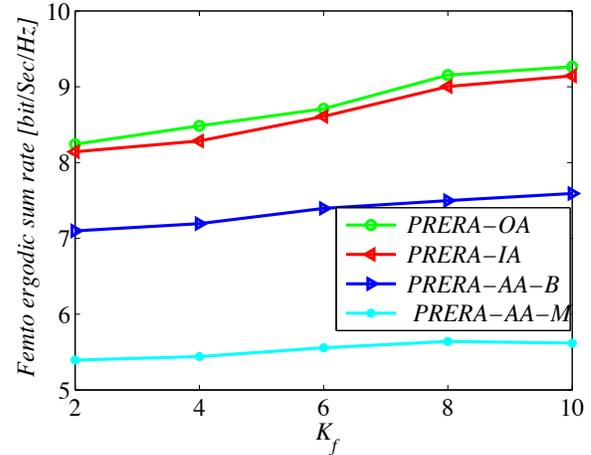
Fig. 2. Femto ergodic sum rate vs.  $K_f$  for PRERA and QPRERA with different levels of quantization.
