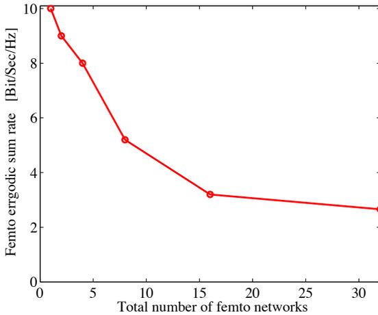
Fig. 6. Femto ergodic sum rate obtained based on QFRERA-IA vs. total number of femto networks.
