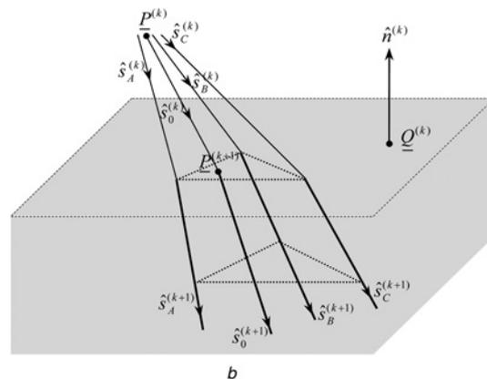
Fig. 3 Interaction of an energy tube with a planar dielectric medium
