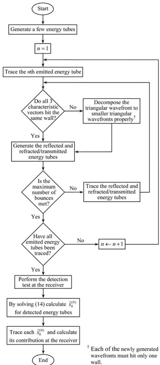
Fig. 6 Flowchart of the modified wavefront decomposition method
