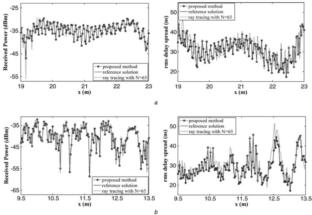
**Fig. 8** Received power and rms delay spread along LOS paths
