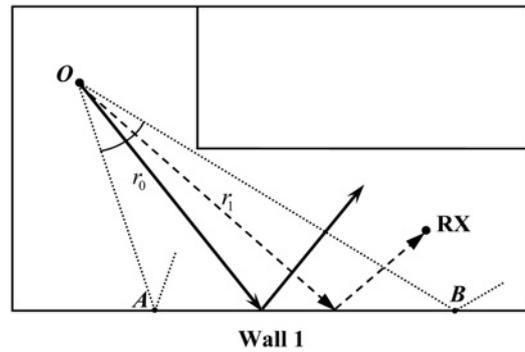
Fig. 2 2D scenario in which the ray  $r_0$  represents the energy tube  $\widehat{AOB}$  and illuminates the receiver location after a single bounce at wall 1
