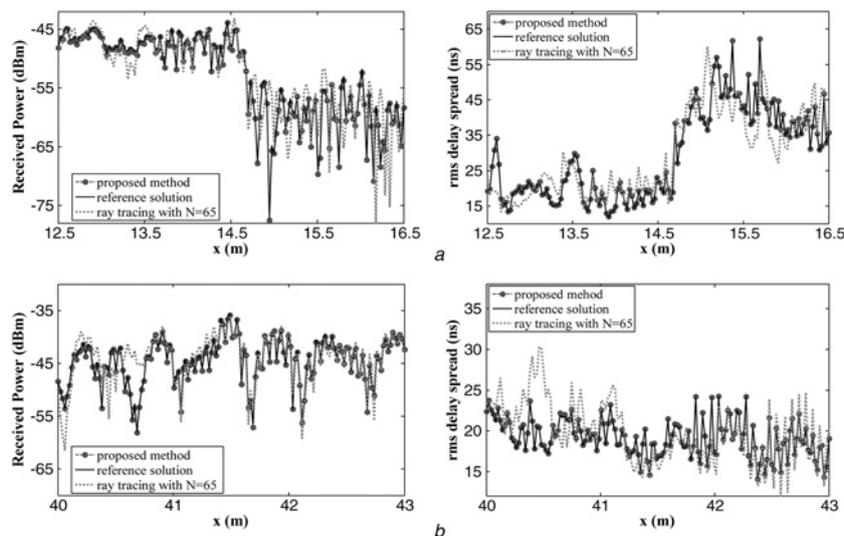
**Fig. 9** Received power and rms delay spread along NLOS paths
