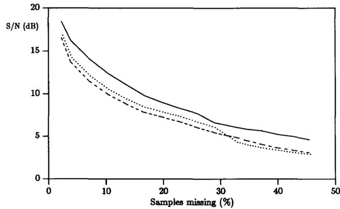
Fig. 5.  $S/N$  results versus percentage loss rate ( $f_s = 8$  kHz). (For comparison see Fig. 3.)
