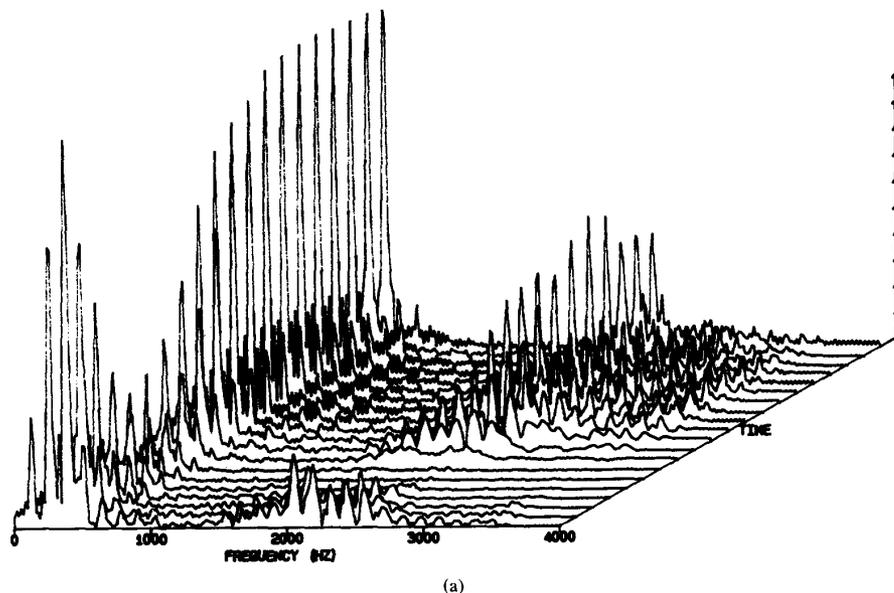
Fig. 4. Time-frequency decomposition of a segment of 1280 samples from the utterance "The navy attacked the big task force."
