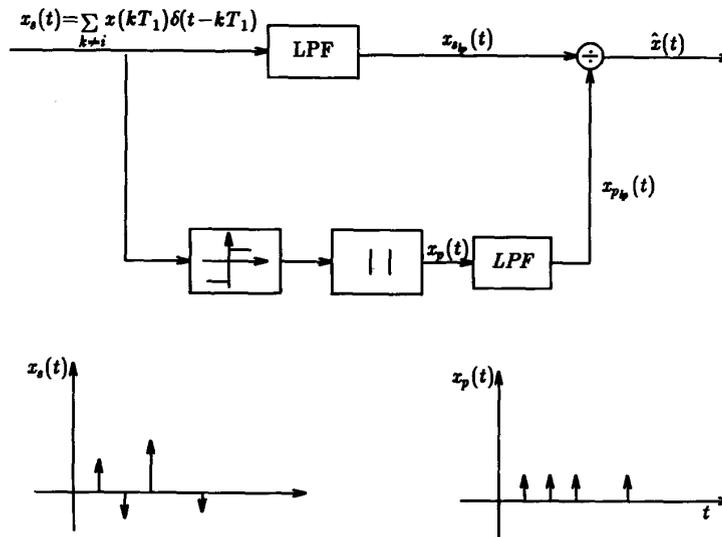
Fig. 1. Block diagram of the reconstruction scheme.
