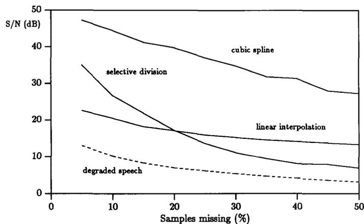
Fig. 6.  $S/N$  results for several interpolation methods ( $f_s = 16$  kHz).
