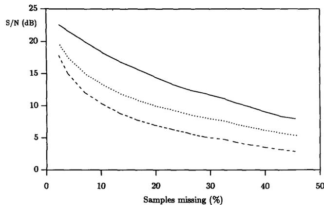
Fig. 3.  $S/N$  results versus percentage loss rate ( $f_s = 16$  kHz). The dashed line represents raw (degraded) speech; the dotted line is the result for low-pass filtering, and the solid line shows the result obtained by processing using the proposed system.
