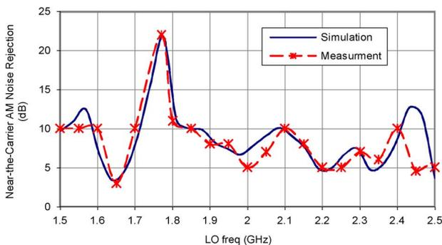
Fig. 10. Near-the-carrier AM noise rejection in branch-line coupler mixer as a function of LO frequency.
