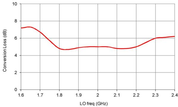
Fig. 8. Conversion loss of rat-race balanced mixer.
