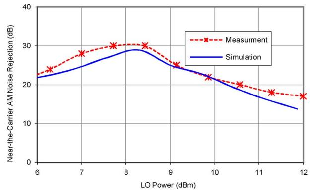
Fig. 11. Near-the-carrier AM noise rejection in branch-line coupler mixer versus LO power for LO frequency of 1.75 GHz.
