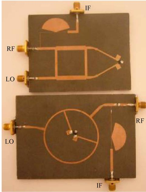
Fig. 4. Fabricated balanced mixers at the center frequency of 2 GHz.
