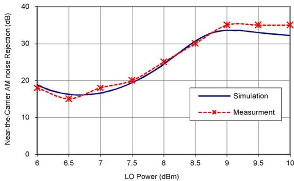
Fig. 9. Near-the-carrier AM noise rejection in rat-race balanced mixer versus the LO Power for LO frequency of 1.85 GHz.
