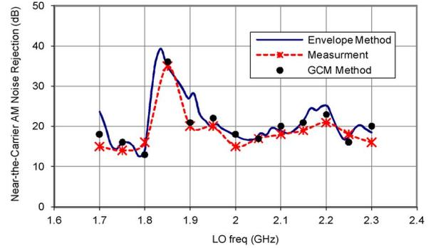
Fig. 6. Near-the-carrier AM noise rejection in rat-race balanced mixer versus the LO frequency.
