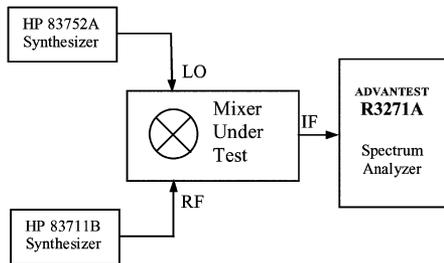
Fig. 5. Measurement setup used.
