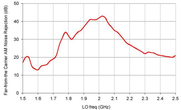
Fig. 7. Far-from-the-carrier AM noise rejection in rat-race balanced mixer.
