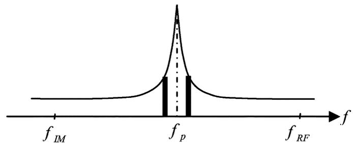
Fig. 2. LO near-the-carrier noise spectrum components.
