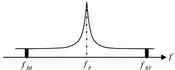
Fig. 1. Far-from-the-carrier LO noise spectrum components.
