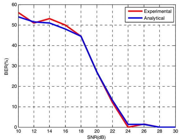
Fig. 5. BER versus SNR for proposed technique, using experimental result and analytical calculations
