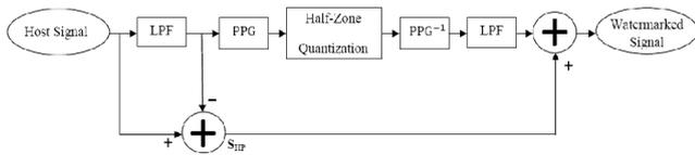
Fig. 6. Block Diagram of Half-Zone Method in the PPG domain
