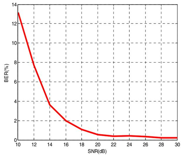
Fig. 7. BER versus SNR, applying proposed technique to an audio signal with noise attack
