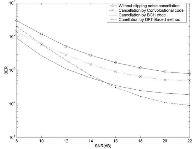
Fig. 8. BER versus SNR for the DFT-Based and the channel coding methods with BW expansion of 1.25 (or coding rate of 4/5)
