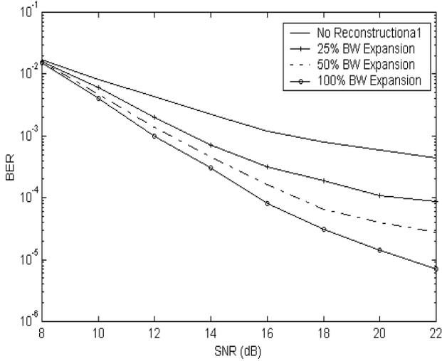
**Fig. 2.** BER versus SNR for PMEPR clipping threshold of 2 and for various BW expansions.
