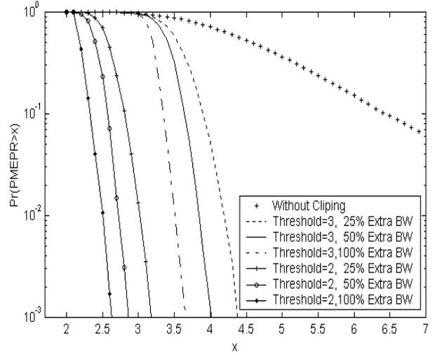
**Fig. 4.** The CCDF of PMEPR after digital clipping and without clipping for various BW expansions.
