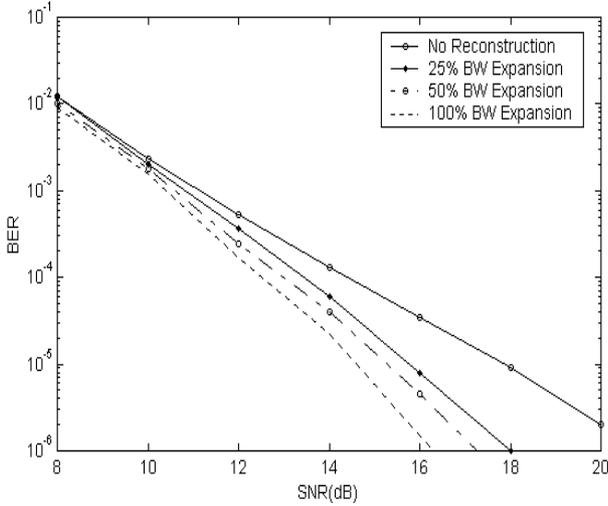
**Fig. 3.** BER versus SNR for PMEPR clipping threshold of 3 and for various BW expansions.
