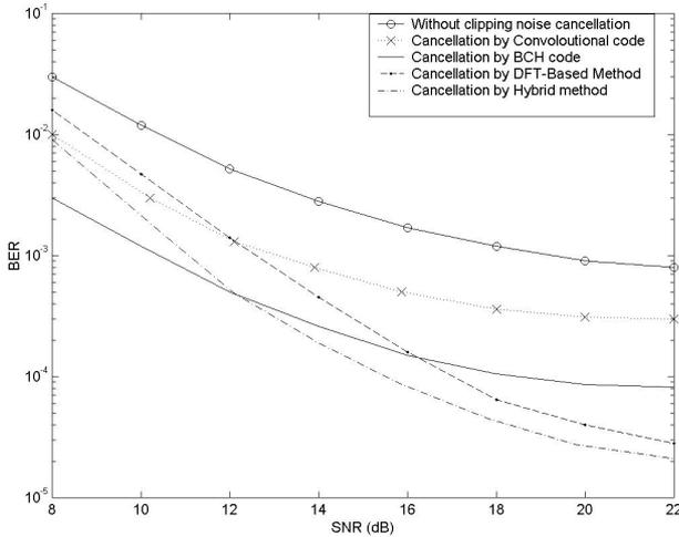
Fig. 7. BER versus SNR for the DFT-Based and the channel coding methods with BW expansion of 1.5 (or coding rate of 2/3)
