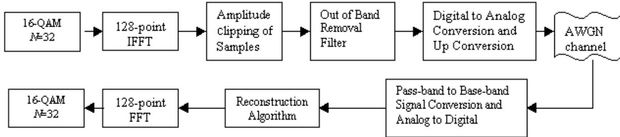
Fig. 1. OFDM transmitter and receiver architecture with digital clipping and DFT-Based Method
