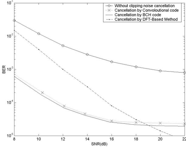
Fig. 6. BER versus SNR for the DFT-Based and the channel coding methods with BW expansion of 2 (or coding rate of 1/2)
