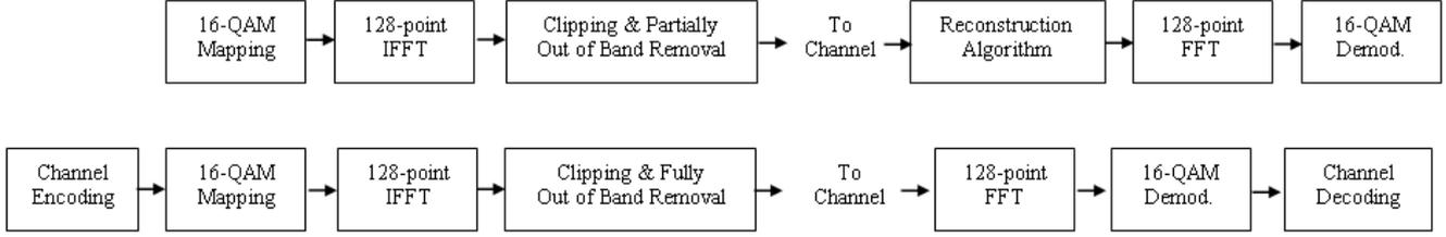
Fig. 5. Block diagrams of transmitter and receiver for the DFT-Based and the channel coding method
