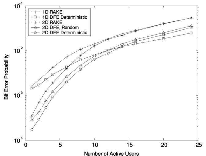
Fig. 4. BEP versus the number of active users at  $E_b/N_0 = 10$  dB ( $L = 3$  paths).
