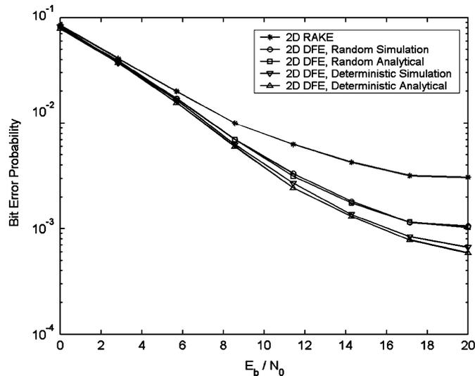
Fig. 3. Receiver BEP versus  $E_b/N_0$  ( $L = 3$  paths and  $K = 8$  users).
