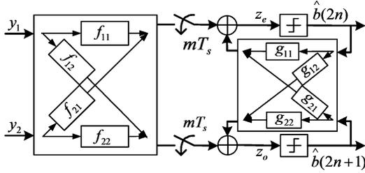
Fig. 2. Space-time coded DFE structure for two transmit antennas.
