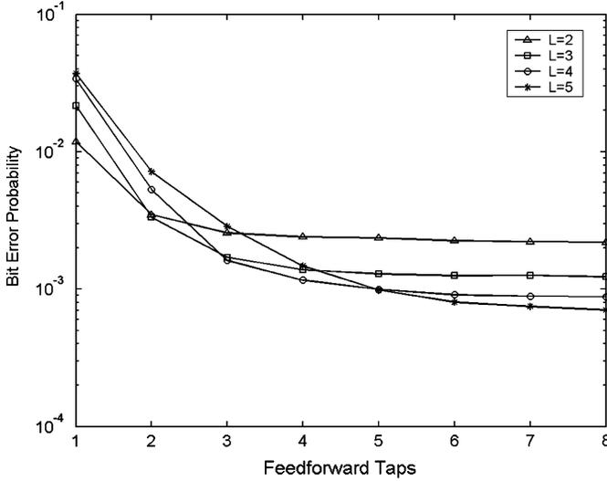
Fig. 5. BEP of deterministic DFE versus  $N_f$  for different values of  $L$  at  $E_b/N_0 = 10$  dB ( $K = 5$  users).
