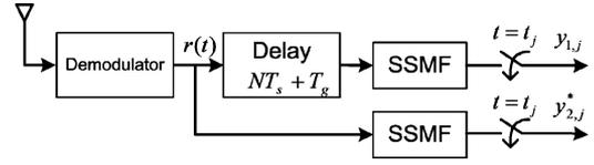
Fig. 1. Preprocessing at the receiver.
