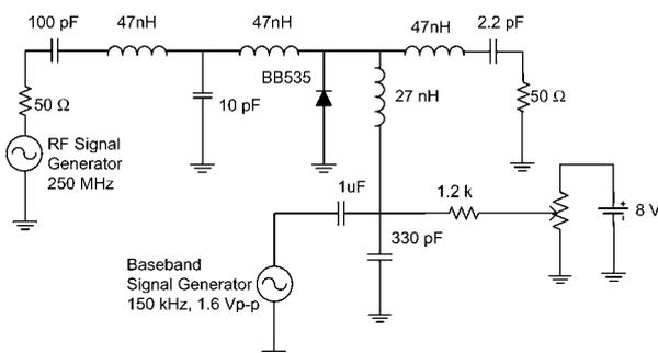
**Figure 8** Schematic of the varactor frequency doubler with the baseband modulating signal applied to the varactor diode
