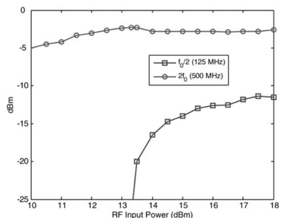
Figure 3 Simulated second harmonic and half frequency output power versus RF input power in the varactor frequency multiplier
