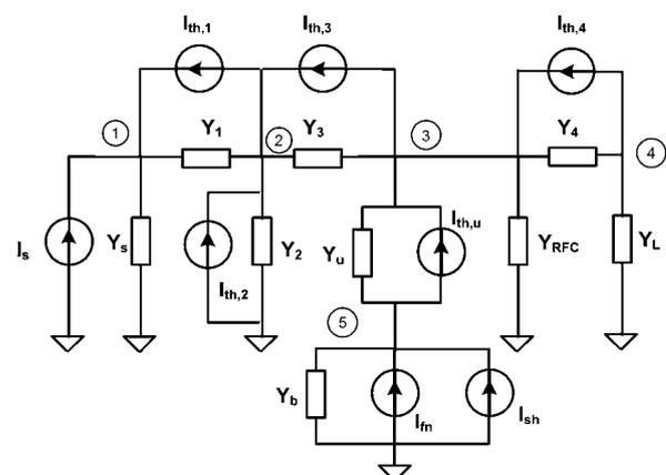
**Figure 2** Small signal circuit of the frequency multiplier used in nodal analysis
