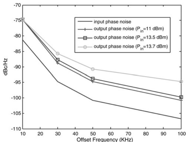
**Figure 6** RF signal generator phase noise spectrum and simulated phase noise spectrum of the frequency doubler for various RF input power levels
