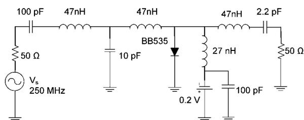
Figure 1 Schematic of the varactor frequency doubler
