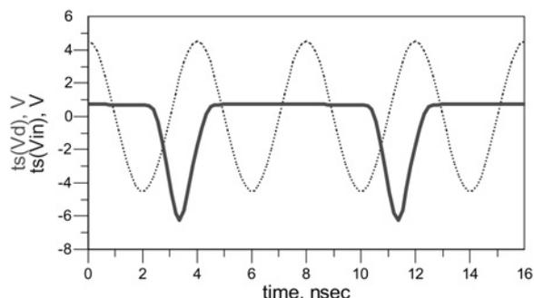
**Figure 4** RF input voltage (dotted line) and diode voltage (continuous line) of the varactor frequency doubler in the presence of subharmonic oscillation
