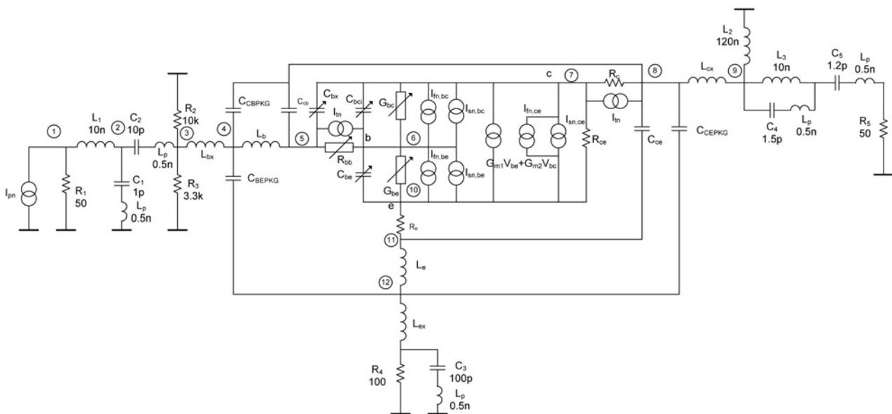
**Figure 12** Linear time variant circuit model of the BJT frequency doubler used in the conversion matrix analysis
