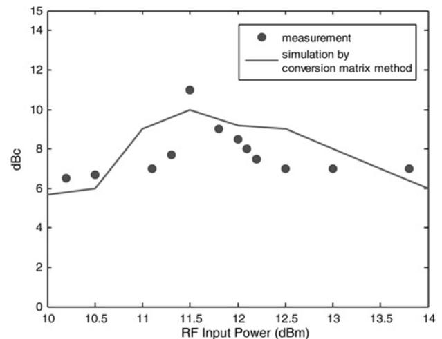
**Figure 15** Relative increase of the output sideband components due to the upconverted baseband signal
