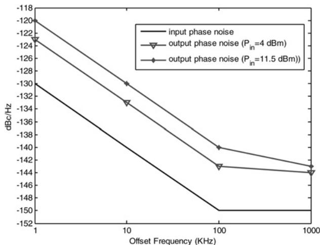
**Figure 13** RF signal generator phase noise spectrum and simulated phase noise spectrum of the BJT frequency doubler for two RF input power levels
