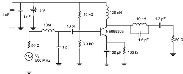
**Figure 10** Schematic of the BJT frequency multiplier
