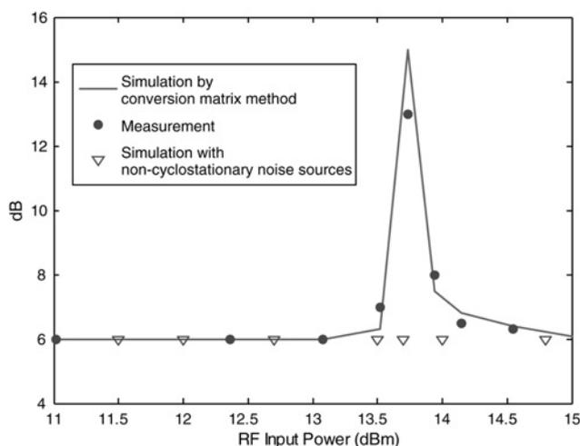
**Figure 5** Output phase noise degradation of the varactor frequency doubler
