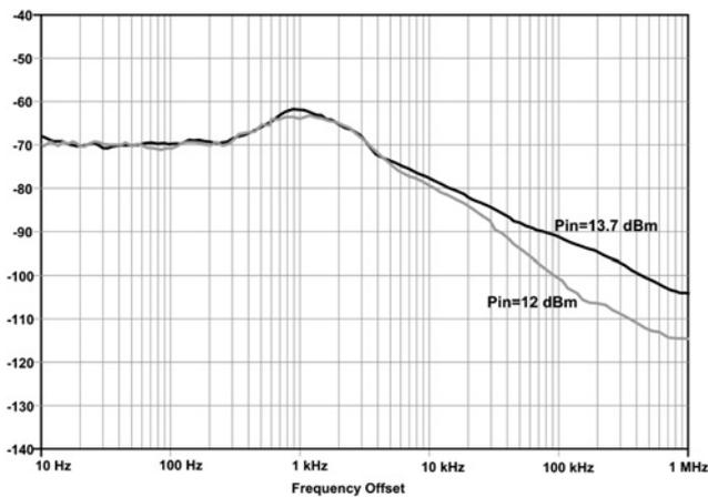
**Figure 7** Measured output phase noise spectrum of the frequency doubler for two RF input power levels
