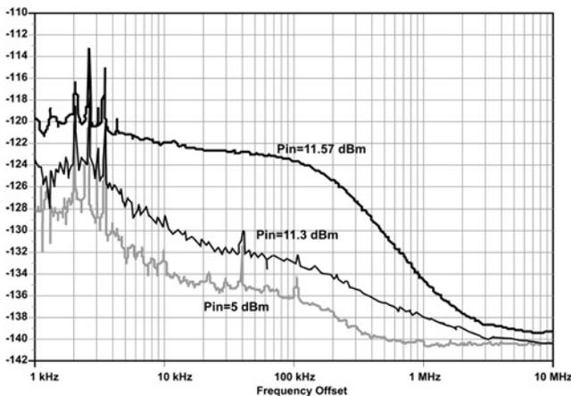
**Figure 14** Measured output phase noise spectrum of the BJT frequency doubler for various RF input power levels
