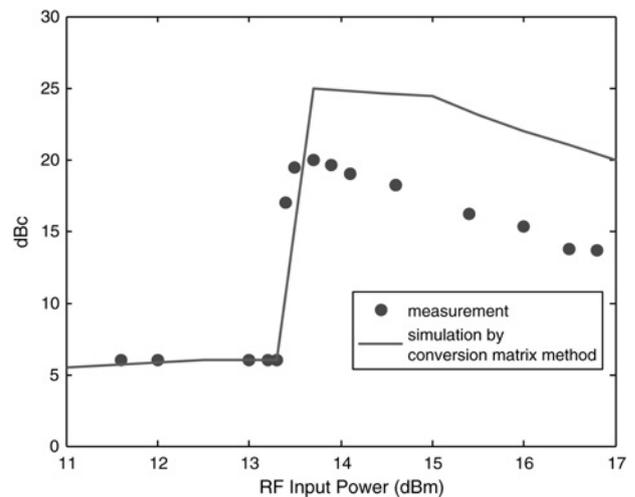
**Figure 9** Increase of the relative power of the output sideband components due to the unconverted baseband signal against input drive
