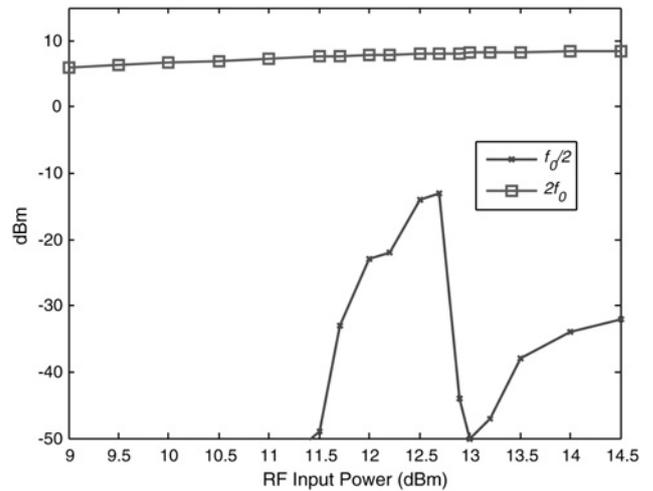
**Figure 11** Simulated second harmonic and half frequency output power against RF input power in the BJT frequency multiplier
