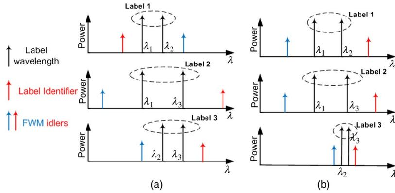
Fig. 1. SAC label recognition by unique LI allocation in (a) an AWG based structure; (b) the proposed FBG based structure.
