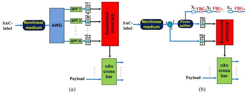
Fig. 8. FWM based SAC label recognition structures: (a) in an AWG based architecture; (b) using our proposed architecture. In both cases  $N$  labels can be generated.
