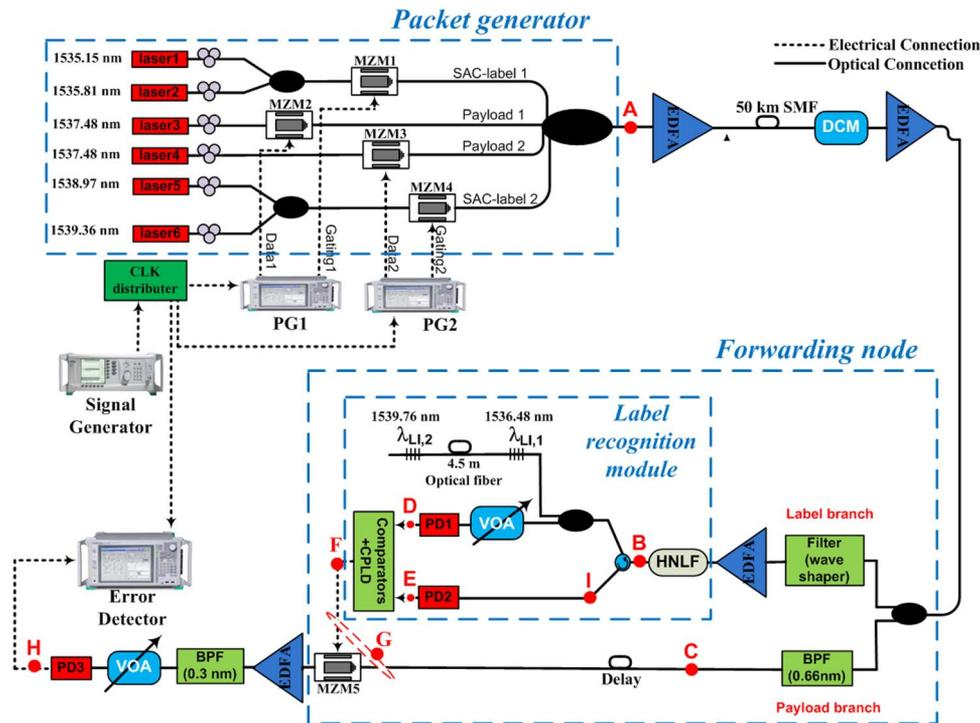
Fig. 3. Experimental setup of the packet switching with SAC-labels. MZM: Mach-Zehnder Modulator, EDFA: Erbium-doped fiber amplifier, DCM: dispersion-compensating module, HNLF: Highly NonLinear Fiber, VOA: Variable Optical Attenuator, BPF: BandPass Filter, PD: PhotoDiode, CPLD: Complex Programmable Logic Device.
