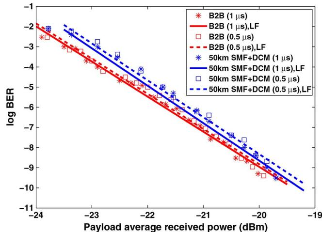
Fig. 7. BER for the payloads of Packets 1 and 2. The solid and dashed lines correspond to the 1 and 0.5  $\mu\text{s}$  payloads, respectively. LF : Linear Fitting.
