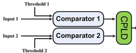
Fig. 6. The schematic of the electronic processing part.
