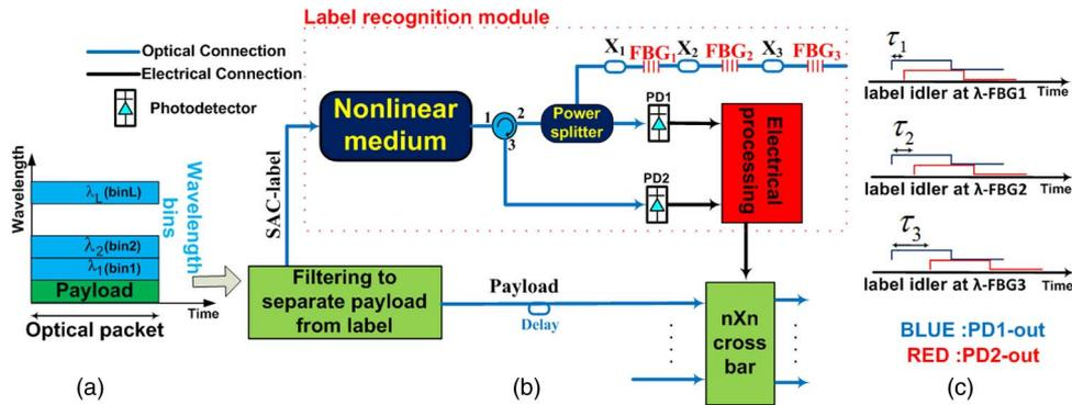
Fig. 2. Schematic diagram of a forwarding node including the proposed SAC label recognition technique (a) optical packet; (b) label recognition module; (c) different characteristic delays for labels.
