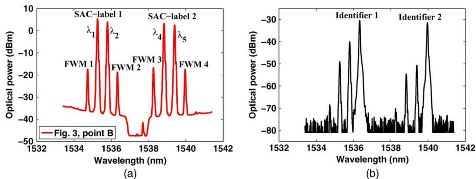
Fig. 5. Optical spectrum analyzer traces of (a) SAC-labels and their FWM idlers, (Fig. 3, point B); (b) FWM idlers reflected back by FBGs (Fig. 3, point I).
