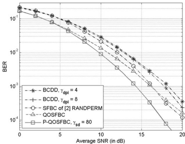
**Fig. 2** BER performance,  $N=1024$ , delay spread  $10 \mu\text{s}$ ,  $2 \text{ bits/s/Hz}$
