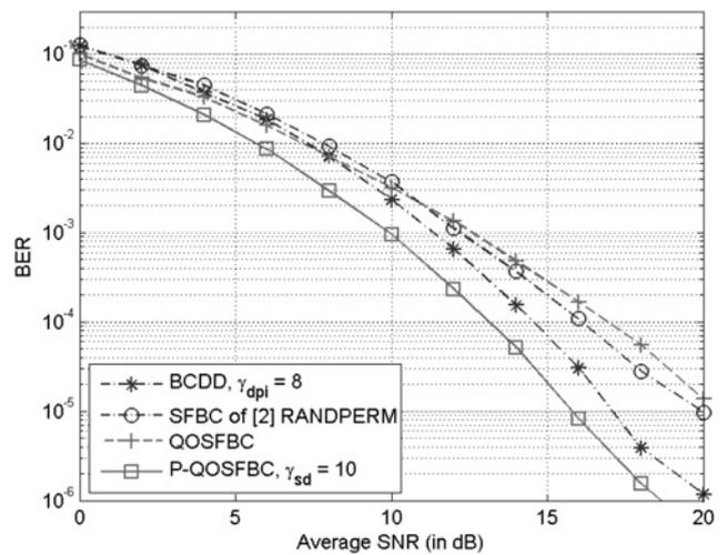
Fig. 1 BER performance,  $N = 128$ , delay spread 5  $\mu$ s, 1 bit/s/Hz
