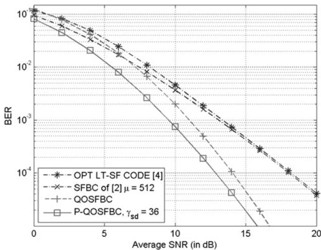
**Fig. 3** BER performance,  $N=1024$ , delay spread  $15 \mu\text{s}$ ,  $1 \text{ bit/s/Hz}$
