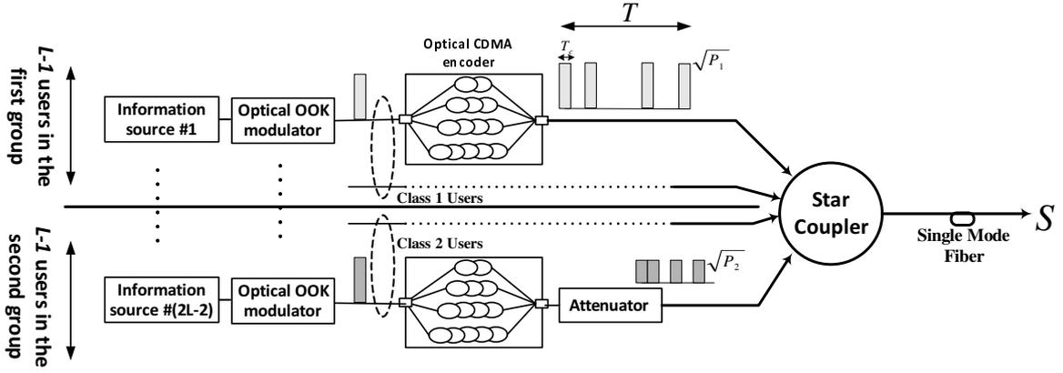
Fig. 1. A schematic diagram of the SOCDMA system based on UWC.
