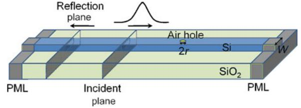
Fig. 2. FDTD simulation structure for the calculation of reflection coefficient. Waveguide section is illuminated by a rib waveguide mode while perfectly matched layer (PML) boundary conditions are used at both ends of the waveguides and reflection coefficient is calculated at indicated plane.
