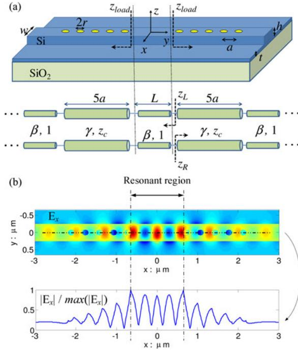
Fig. 4. (a) Schematic view of a typical Fabry-Perot PCNBR together with its equivalent TL model. (b) The  $x$  component of the electric field profile ( $E_x$ ) of the resonance mode extracted from FDTD and absolute value of  $E_x$  in  $x = 0$  along the resonator.
