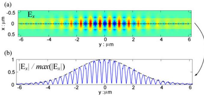
Fig. 7. (a) A snapshot of the  $x$  component of the electric field profile ( $E_x$ ) of the resonance mode extracted from 3-D FDTD for a PCNBR with photonic crystal waveguide mirrors that are composed of 15 unit cells. (b) The absolute value of  $E_x$  in  $x = 0$  along the resonator (blue solid line) and a Gaussian distribution with the standard deviation of  $\sigma = 2 \mu\text{m}$  (dashed-dotted black line).
