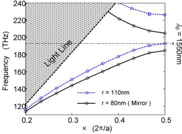
Fig. 5. Band structure of the photonic crystal waveguide mirrors with  $r_m = 80$  nm (black solid lines), and the innermost photonic crystal waveguide section with  $r_1 = 110$  nm (blue dashed lines). These values are chosen to make sure that the desired communication wavelength 1550 nm will be at the center of the photonic gap of PC waveguide mirror and at the band edge of innermost PC waveguide sections.
