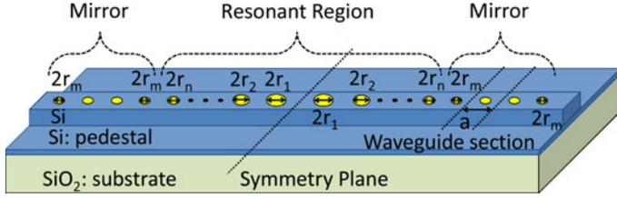
Fig. 1. Schematic view of a typical silicon PCNBR.
