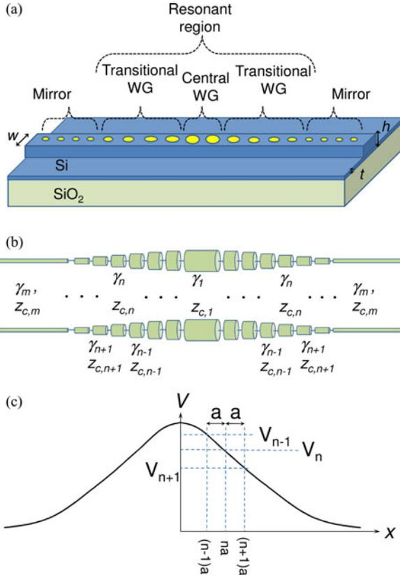
Fig. 6. (a) Schematic view of the PCNBR. (b) TL model of the PCNBR. (c) The desired Gaussian voltage distribution.
