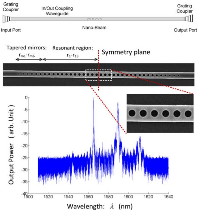
Fig. 8. Direct coupling scheme, characterization curve, and SEM image of the direct coupled nano-beam.
