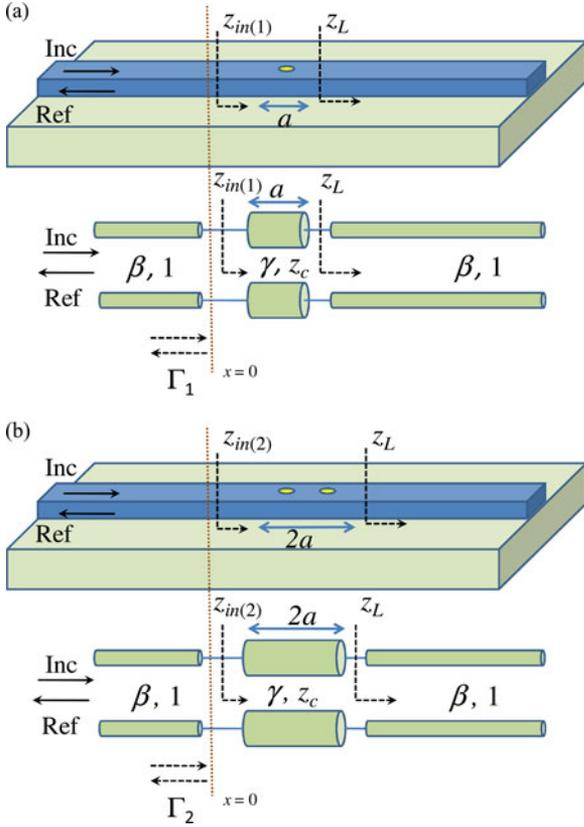
Fig. 3. Extraction of the TL model for a typical waveguide section of the PCNBR shown in Fig. 1. (a) The first step in extraction of the model parameters. (b) The second step in extraction of the model parameters.
