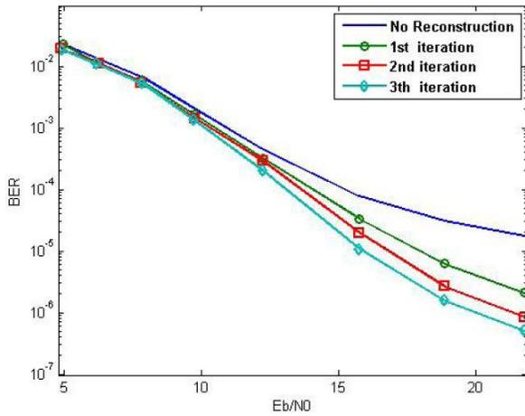
Fig. 6. BER versus  $\frac{E_b}{N_0}$  with decorrelator, clipping ratio of  $\gamma = \sqrt{2}$ , Number of users  $L=17$ , SIR=-12.04 dB.
