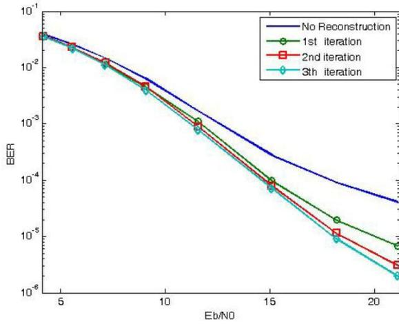
Fig. 5. BER versus  $\frac{E_b}{N_0}$  with decorrelator, clipping ratio of  $\gamma = \sqrt{2}$ , Number of users  $L=20$ , SIR=-12.79 dB.
