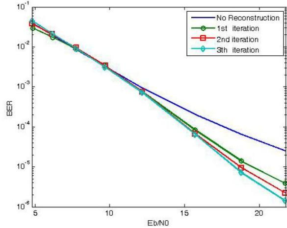
Fig. 4. BER versus  $\frac{E_b}{N_0}$  with decorrelator, clipping ratio of  $\gamma = \sqrt{3}$ , Number of users  $L=23$ ,  $SIR=-13.4$  dB.
