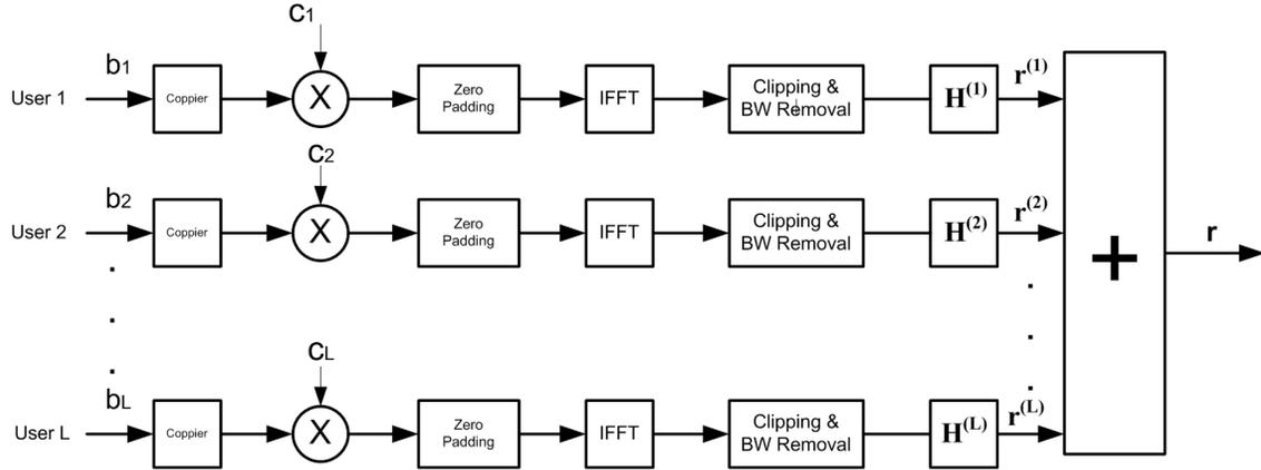
Fig. 1. The Block Diagram of an uplink MC-CDMA system,  $\mathbf{r}$  is received signal in base-station.
