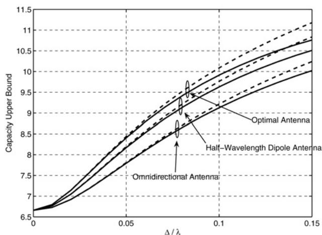
**Figure 5** Jensen upper bound (solid curves) and its approximation (dashed curves) against the normalised distance between antennas
