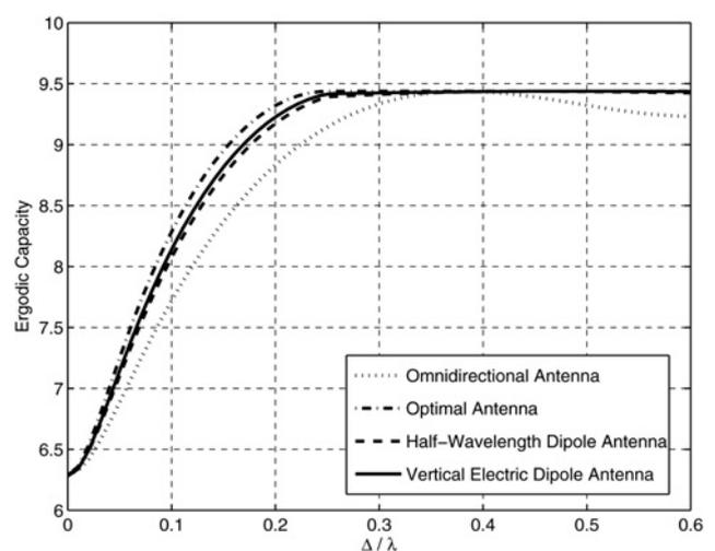
**Figure 4** Ergodic capacity for four cases: omnidirectional antenna, the optimal antenna, the half-wavelength dipole and the vertical electric dipole with the size of  $L = 0.2\lambda$  against the normalised distance of the antennas
