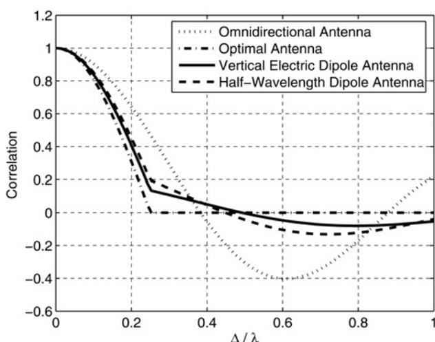
**Figure 2** Behaviour of correlation factor for four cases: omnidirectional antenna, the optimal antenna, half-wavelength dipole and the vertical electric dipole with the size of  $L = 0.2\lambda$  against the distance of the antennas normalised with respect to the wavelength
