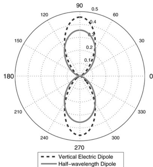
**Figure 3** Antenna pattern for the half-wavelength dipole and the vertical electric dipole
