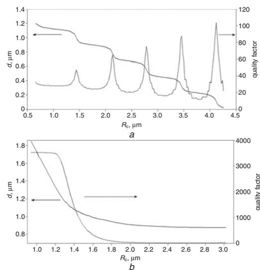
**Fig. 2** Thickness (solid line) and quality factor (dashed line) of typical homogeneous ring with  $TE_{0,6}$ , and  $TE_{11,4}$  resonance wavelength  $\lambda = 1.55 \mu\text{m}$  against average radius of ring
