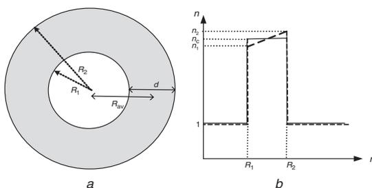
**Fig. 1** Schematic of micro-ring resonator, and refractive index profiles of homogenous and linearly homogeneous ring resonator
