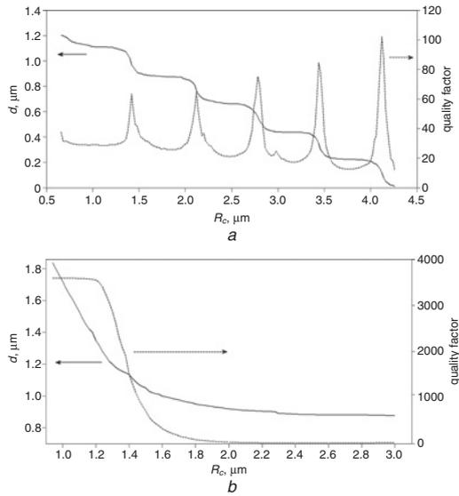
**Fig. 3** Thickness (solid line) and quality factor (dashed line) of typical inhomogeneous ring with  $TE_{0,6}$ , and  $TE_{11,4}$  resonance wavelength  $\lambda = 1.55 \mu\text{m}$  against average radius of ring
