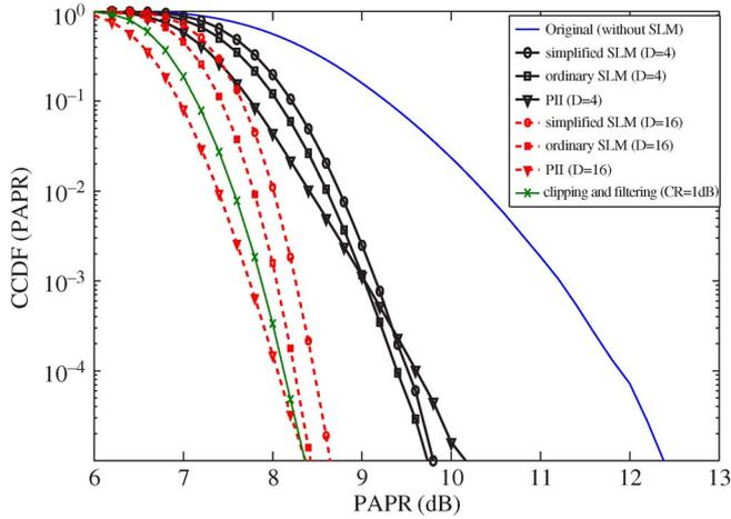
Fig. 2. PAPR reduction performance of the ordinary SLM, simplified SLM, PII, and clipping and filtering methods for the SFBC-OFDM system with two transmitter antennas and  $N_c = 128$  for different values of  $D$ .
