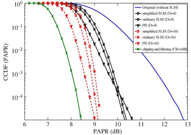
Fig. 3. PAPR reduction performance of the ordinary SLM, simplified SLM, PII, and clipping and filtering methods for the SFBC-OFDM system with two transmitter antennas and  $N_c = 512$  for different values of  $D$ .
