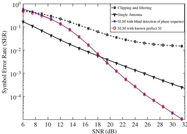
Fig. 5. SER performance of the SFBC-OFDM system with two transmitter antennas and  $N_c = 512$  with three different PAPR reduction methods. 1) Simplified SLM with perfect SI ( $D = 16$ ); 2) simplified SLM ( $D = 16$ ) with blind detection of SI; and 3) clipping and filtering, and SER performance of a single-antenna OFDM system.
