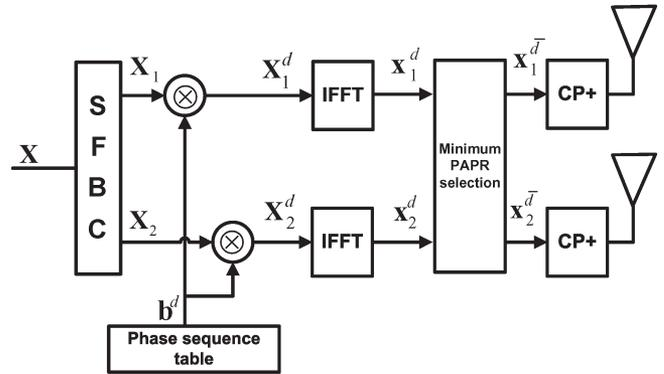
Fig. 1. Block diagram of the SFBC-OFDM transmitter with two transmitter antennas and the SLM method for PAPR reduction.
