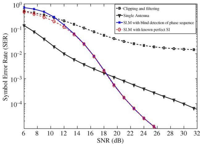
Fig. 4. SER performance of the SFBC-OFDM system with two transmitter antennas and  $N_c = 128$  with three different PAPR reduction methods. 1) Simplified SLM with perfect SI ( $D = 16$ ); 2) simplified SLM ( $D = 16$ ) with blind detection of SI; and 3) clipping and filtering, and SER performance of a single-antenna OFDM system.
