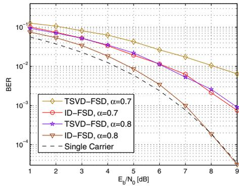
Fig. 4. BER performance for ID-FSD and TSVD-FSD detectors carrying 4QAM symbols for  $N=16$ ,  $v=20$  for  $T_W=16$ .
