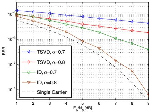
Fig. 3. BER performance for ID and TSVD detectors carrying 4QAM symbols for  $N=16$ ,  $v=20$  for  $T_W=16$  with  $\alpha = 0.7$  and  $0.8$ .
