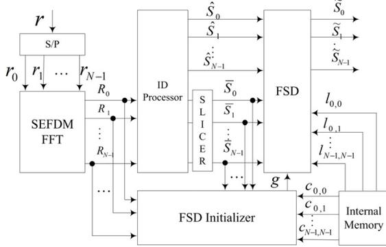
Fig. 2. Block diagram of ID-FSD detector.
