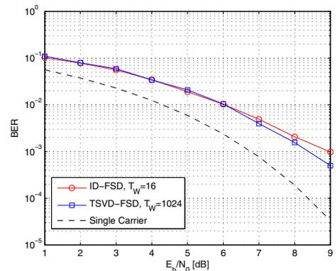
Fig. 5. BER performance for different detectors carrying 4QAM symbols for  $N=16$ ,  $v=20$ ,  $\alpha=0.7$ .
