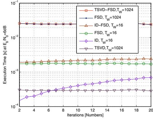
Fig. 6. Execution time versus iteration numbers for different SEFDM detectors carrying 4QAM symbols with  $\alpha = 0.7, N=16$ .
