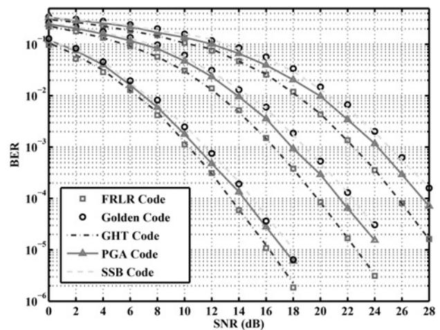
**Fig. 3** BER performance comparison between different STBCs for the PAM constellation
