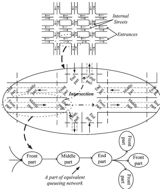
Fig. 1. Typical roadmap (road topology) considered in this paper and the method of mapping different parts of the streets onto queueing nodes.
