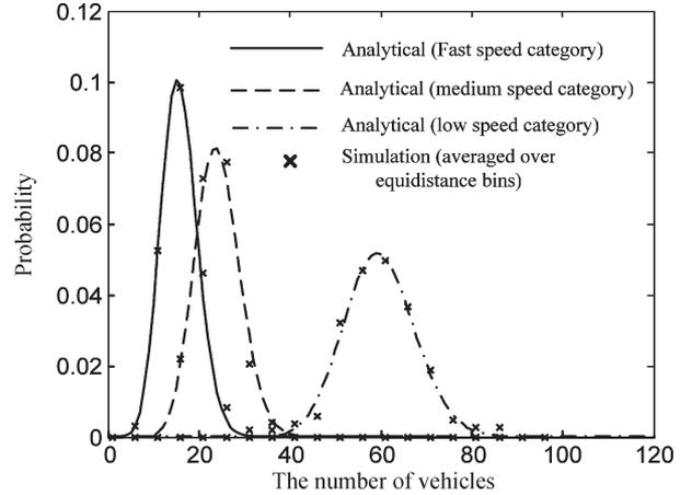
Fig. 6. Stationary probability distribution (state-independent model) for the number of vehicles with different speed categories in the middle part of a typical street in the case of uniform mobility pattern ( $\lambda = 0.8$  vehicles/s).
