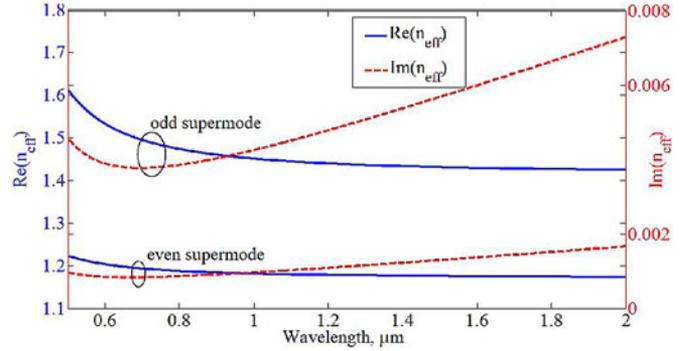
Fig. 2. Effective refractive indices of even and odd supermodes versus the wavelength of light at free space. The geometrical parameters are in accordance with Fig. 1:  $w_1 = 60$  nm,  $w_2 = 10$  nm, and  $d = 20$  nm.
