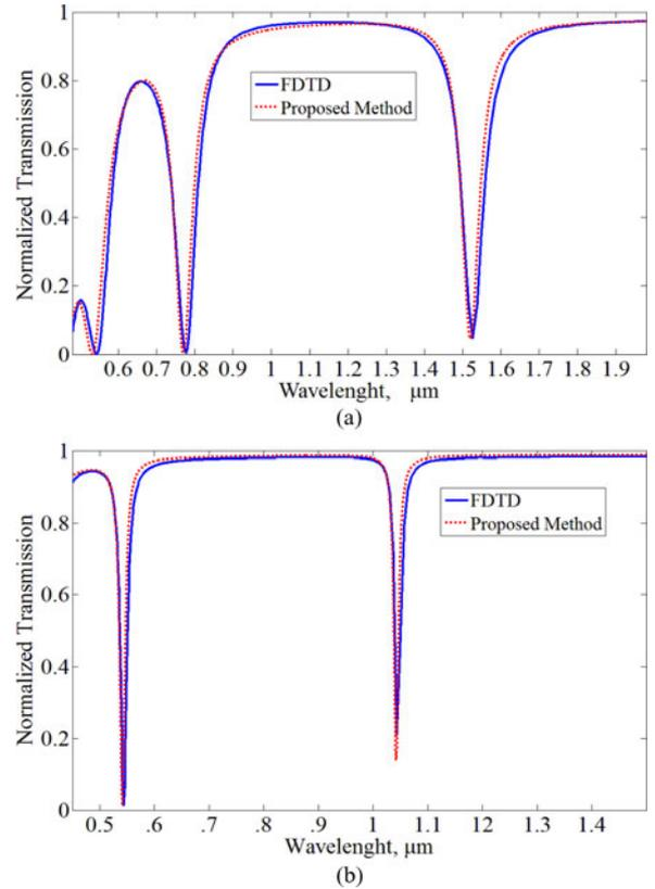
Fig. 5. (a) Transmission spectrum of a side-coupled resonator with  $w_1 = 50$  nm,  $w_2 = 50$  nm,  $h = 20$  nm, and  $d = 500$  nm [7]: the FDTD results (solid line), and the proposed circuit model (dashed line). (b) Transmission spectrum of a side-coupled resonator with  $w_1 = 60$  nm,  $w_2 = 120$  nm,  $h = 32$  nm, and  $l = 400$  nm: the FDTD results and (solid line), the proposed method (dashed line).
