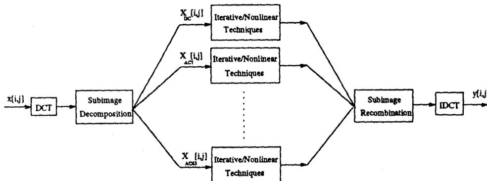
Figure 4: A general block diagram of the subimage error concealment technique.
