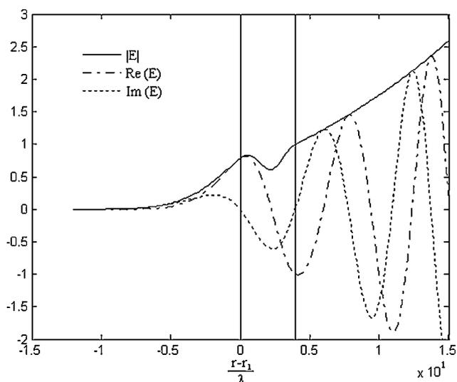
**Figure 7** Electrical wavefunction of second mode against  $r - r_1$  with  $\alpha_1 = \alpha_2 = 0$ ,  $\beta_2/k_0 = 1.4972 - 1.814 \times 10^{-3}i$
