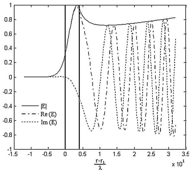
**Figure 3** Electrical wavefunction of first mode against  $r-r_1$  with  $\alpha_1 = \alpha_2 = 0$ ,  $\beta_1/k_0 = 1.5021 - 4.725 \times 10^{-4} i$ . Inner and outer boundaries are shown by using solid lines
