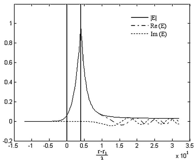
**Figure 4** Electrical wavefunction of first mode against  $r-r_1$  with  $\alpha_1 = 0$ ,  $\alpha_2 = -0.2$ ;  $\beta_1/k_0 = 1.5064 - 5.386 \times 10^{-6} i$
