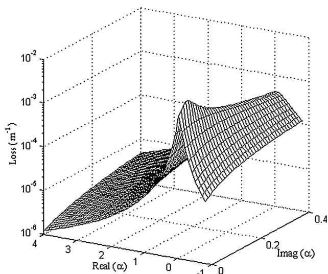
**Figure 6** Loss against real and imaginary parts of  $\alpha$  for the second leaky mode
