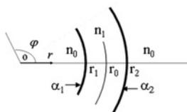
Figure 1 Bent waveguide with central radius  $r_0$
