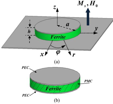
Fig. 1. (a) Geometry of the normally magnetized ferrite disk. (b) Analytical model structure with PMC sidewall approximation.
