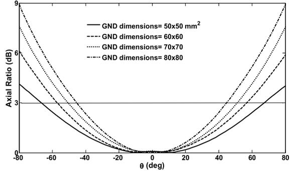
Fig. 7. Full-wave AR pattern at the resonance frequency ( $f = 4.225$  GHz) for different ground dimensions. The other design parameters are the same as in Fig. 4.
