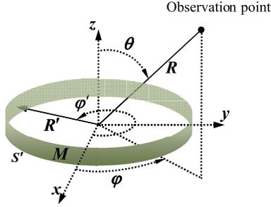
Fig. 2. Equivalent magnetic surface current model for the magnetized ferrite disk structure shown in Fig. 1.
