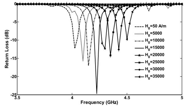
Fig. 9. Full-wave simulated of the return loss against the magnetic bias field. The other design parameters are the same as in Fig. 4.
