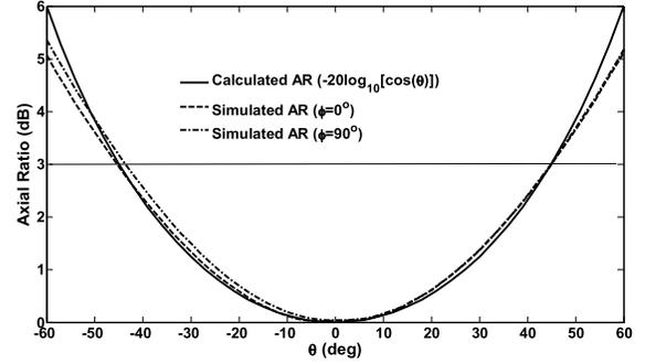
Fig. 6. Comparison of theoretical and full-wave simulation results for AR pattern at the resonance frequency. The design parameters are the same as in Fig. 4.
