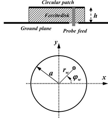
Fig. 3. Cross sectional (top) and top view (bottom) of the ferrite disk with the current probe feed at  $r_w, \varphi_w$ .
