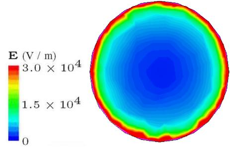
Fig. 5. Electric field distribution computed by HFSS along the circular patch at the resonance frequency. The design parameters are the same as in Fig. 4.
