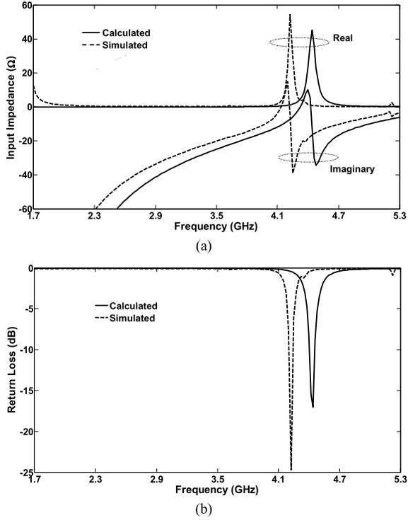
Fig. 4. Comparison of theoretical and full-wave simulation results for (a) antenna input impedance and (b) return loss. The frequency range is  $\omega_{\perp} < \omega < \omega_H + \omega_M \cdot a = 5$  mm,  $r_w = 2.1$  mm,  $h = 1$  mm,  $H_0 = 15000$  A/m, and the ground dimensions =  $80 \times 80$  mm<sup>2</sup>.
