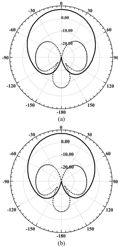
Fig. 8. Circularly polarized radiation patterns at the resonance frequency, the design parameters are the same as in Fig. 4. Dashed line: right-hand circularly polarized pattern. Solid line: left-hand circularly polarized pattern. (a)  $x$ - $z$  and (b)  $y$ - $z$  plane.
