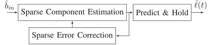
Fig. 2. Block diagram for reconstruction at the receiver.
