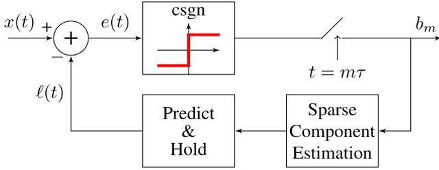
Fig. 1. Block diagram for the proposed acquisition scheme.
