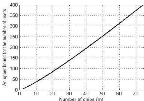
Figure 1. The upper bound of Theorem 6 for the number of users versus the number of chips.
