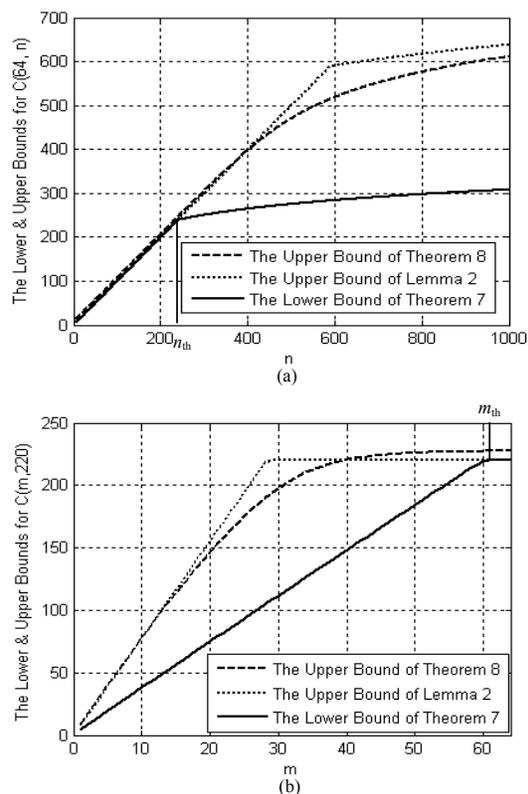
Figure 2. Lower and upper bounds for the sum channel capacity with respect to: (a) the number of users  $n$  for  $m = 64$ , (b) the chip rate  $m$  for  $n = 220$ .
