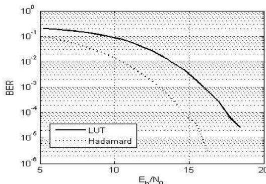
Figure 4. Bit-error-rate versus  $E_b/N_0$ . The dashed curve is a Hadamard code with 64 chips and 64 users. The solid curve is the table look up method for a COW code with 64 chips and 104 users.
