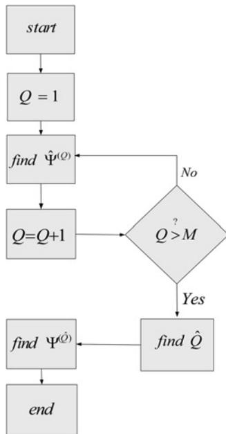
Fig. 4 Flowgraph of the proposed spectrum-sensing method
