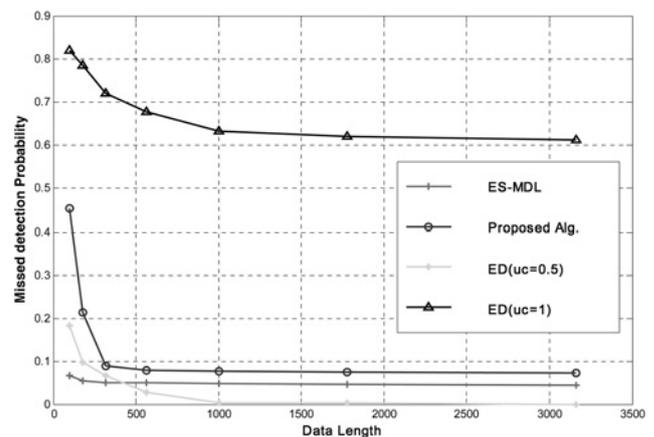
**Fig. 8** Missed detection probability against different data lengths (sensing time),  $M = 6$ ,  $Q = 3$  and  $SNR = 5$  dB
