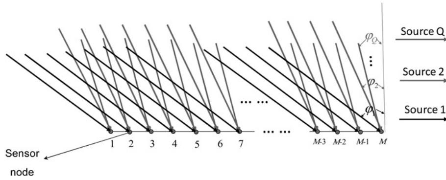
Fig. 2 Illustration of DOA estimation with  $M$  sensor nodes and  $Q$  users' signals
