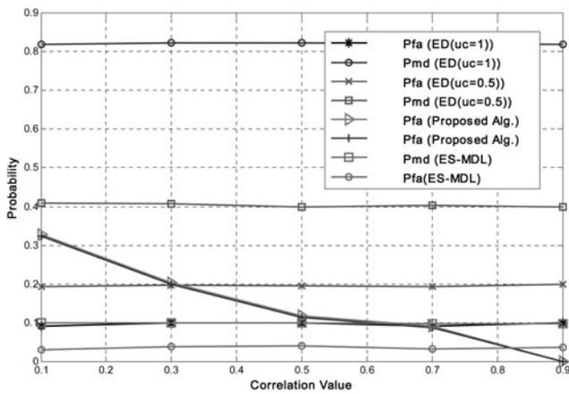
Fig. 10 Missed detection and false alarm probabilities against different correlation values,  $M = 6$ ,  $Q = 3$  and  $SNR = 0$  dB
