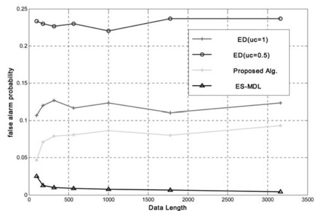
**Fig. 9** False alarm probability against different data lengths (sensing time),  $M = 6$ ,  $Q = 3$  and  $SNR = 5$  dB
