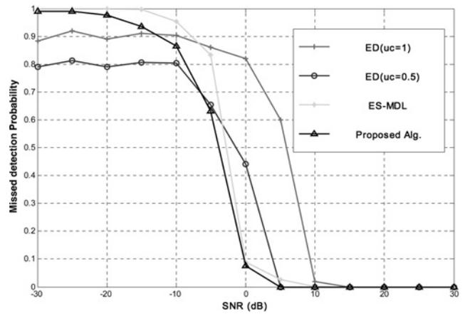
Fig. 5 Missed detection probability against SNR,  $M = 6$  and  $Q = 3$
