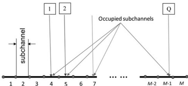
Fig. 1 Illustration of the wideband spectrum sensing for  $M$  subchannels and  $Q$  occupied subchannels
