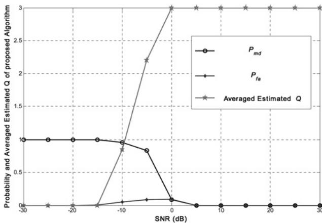
**Fig. 7** Missed detection probability, false alarm probability and average estimated  $Q$  against different SNR values in the proposed algorithm,  $M = 6$  and  $Q = 3$
