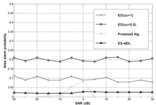
Fig. 6 False alarm probability against different SNR values,  $M = 6$  and  $Q = 3$
