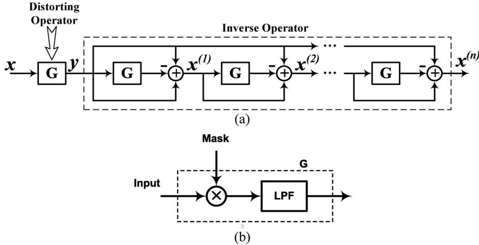
Fig. 3. (a) Block diagram of the iterative method with  $\lambda = 1$ . (b) Model of the distortion block  $G$  in our specific application.
