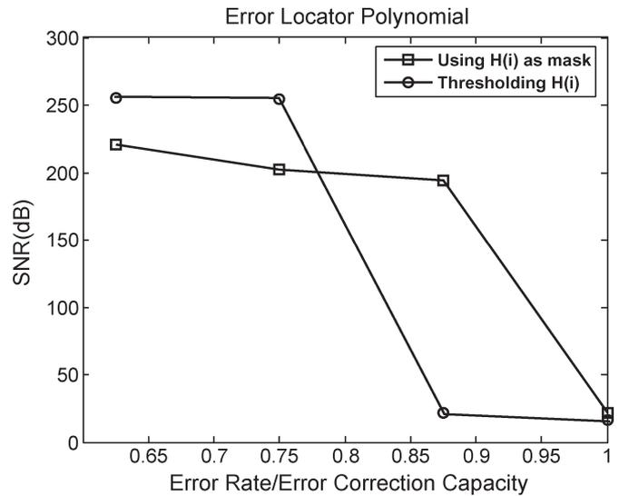
Fig. 7. SNR of the denoised signal using ELP to generate mask.
