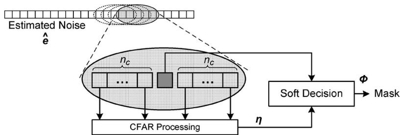
Fig. 2. Typical CFAR detector and decision block.
