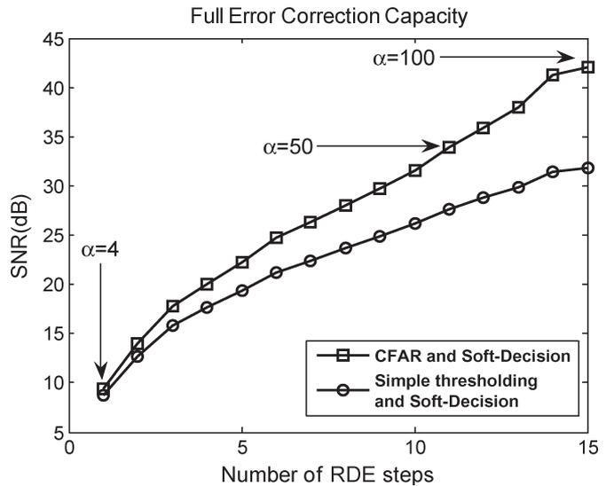
Fig. 5. Comparison of CFAR and simple soft decision at full capacity.
