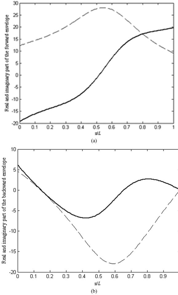
Fig. 3. (a) Real (solid line) and imaginary (dashed line) parts of the normalized  $A^+(z)$ , i.e., forward envelope function versus normalized coordinate in nonlinear region. (b) Real (solid line) and imaginary (dashed line) parts of the normalized  $A^-(z)$ , i.e., backward envelope function versus the normalized coordinate in the nonlinear region.
