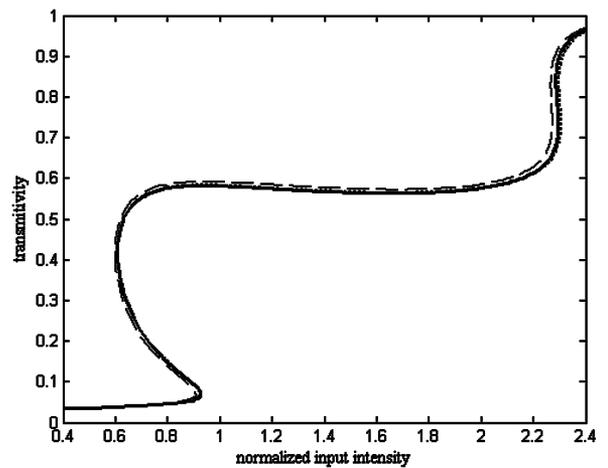
Fig. 4. Transmittivity versus the normalized input intensity: RK2 with 1500 intervals (dotted line), RK4 with 1000 (solid line) and 500 intervals (dashed line) applied to the proposed WKB factorization technique.
