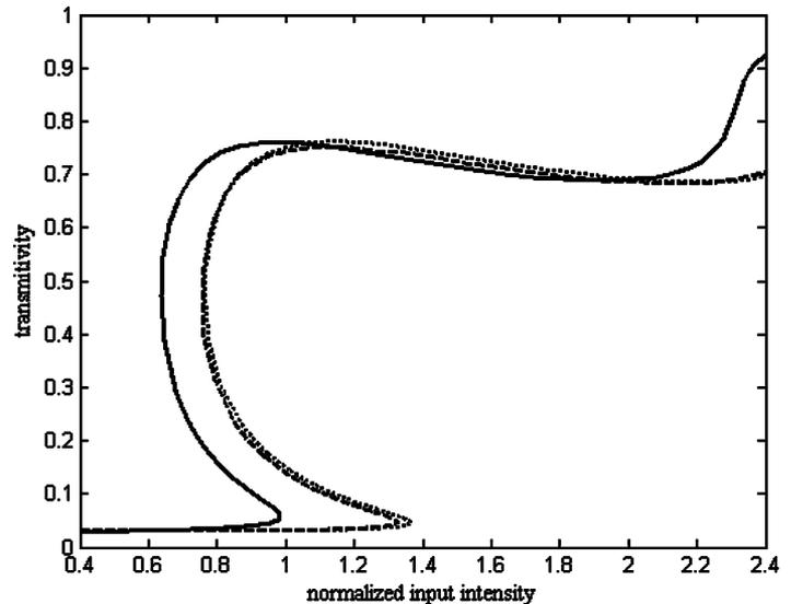
Fig. 7. Transmittivity versus the normalized input intensity: Adams-Bashforth-Moulton (solid line), Gear's method (dashed line) and Rosenbrock formula of order 2 (dotted line) applied to the Maxwell's equations [11].
