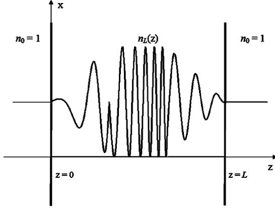
Fig. 1. Schematic of the considered NLDFB with arbitrary refractive index profile  $n_L(z)$ .
