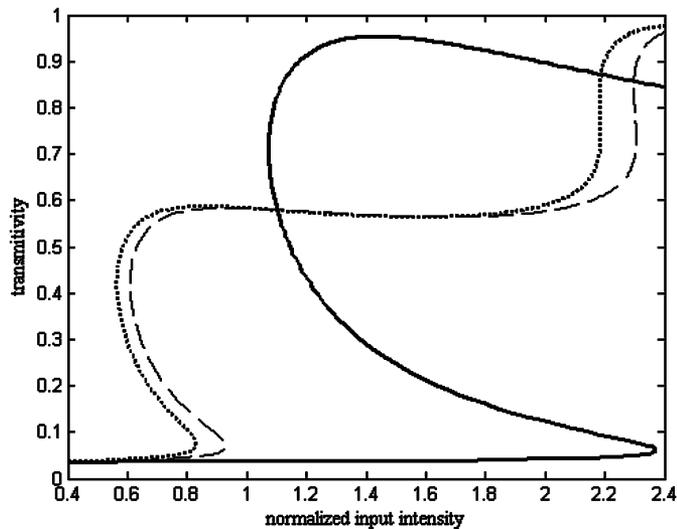
Fig. 5. Transmittivity versus the normalized input intensity: RK2 with 30000 intervals (dotted line), RK4 with 1000 (solid line) and 3000 intervals (dashed line) directly applied to the Maxwell's equations [11].
