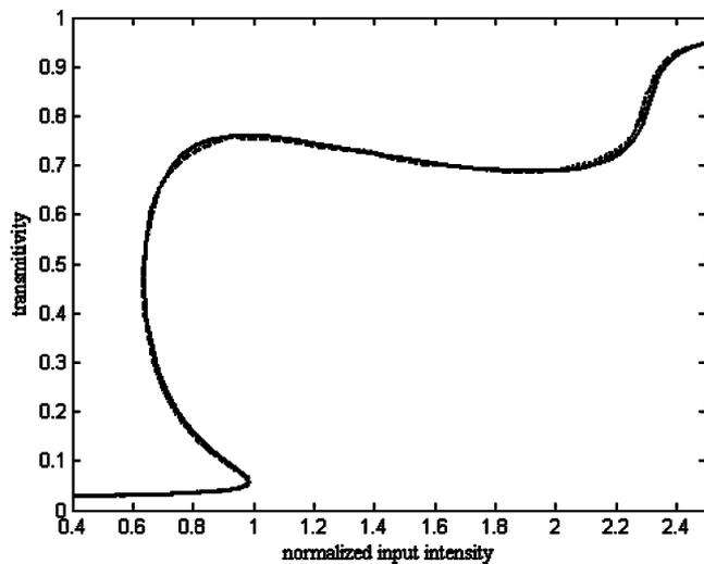
Fig. 6. Transmittivity versus the normalized input intensity: Adams-Bashforth-Moulton (solid line), Gear's method (dashed line) and Rosenbrock formula of order 2 (dotted line) applied to the proposed WKB factorization technique.
