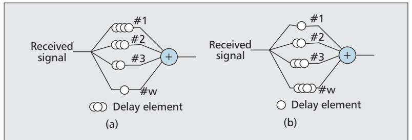
Figure 1. a) An all-optical encoder; b) An all-optical decoder.
