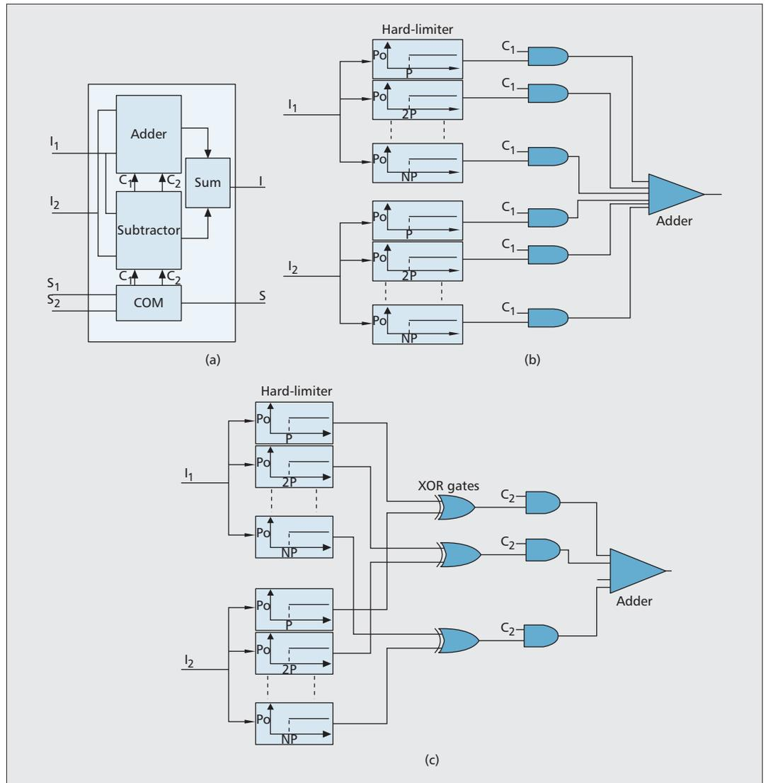
**Figure 3.** a) The block diagram of the adder/subtractor; b) the block diagram of an all-passive optical adder; c) the block diagram of an all-passive optical subtractor.
