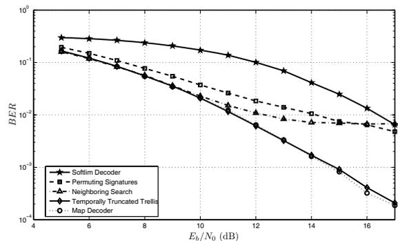
Fig. 2. BER for the proposed sub-optimum decoders.
