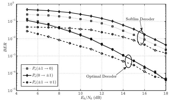
Fig. 1. Probability of error for the three possible kinds of errors for the proposed MAP decoder and the previous best decoder (Softlim).
