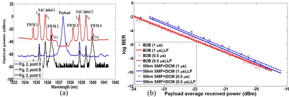
Fig. 3. a) Optical spectrum analyzer traces of SAC labels and their FWM idlers, as well as the extracted payload, and FWM idlers reflected back by FBGs, b) BER versus average received power for back-to-back, and after 50 km of SMF with DCM. LF: Linear fitting.
