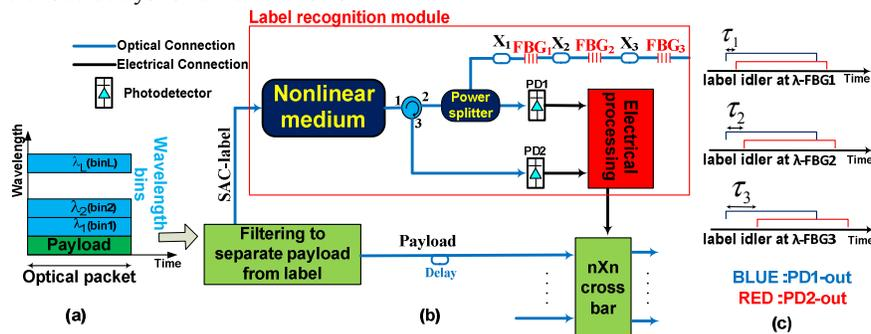
Fig. 1. a) Optical packet with SAC labels, b) structure of the forwarding node, c) different delays between two signals for different labels.
