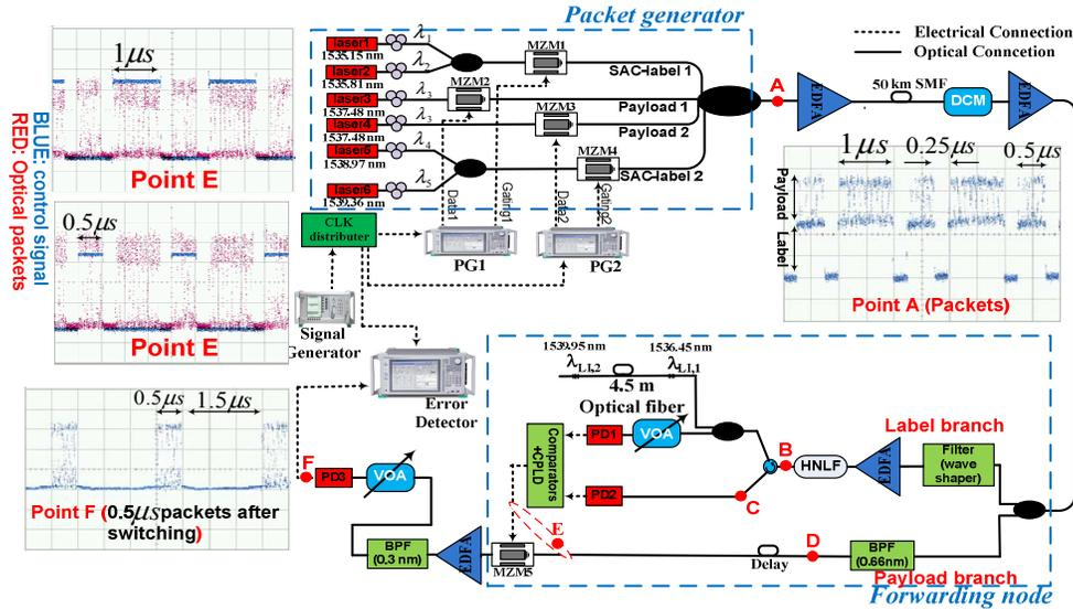
Fig. 2. Experimental setup of the packet switching with SAC-labels, with insets showing the recorded waveform at various points. MZM: Mach Zehnder Modulator, EDFA: Erbium-doped fiber amplifier, DCM: dispersion-compensating module, VOA: Variable Optical Attenuator.
