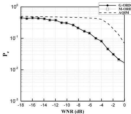
**Fig. 3.** Comparing the probability of error with DWR=19dB between our method and the AQIM method [8]
