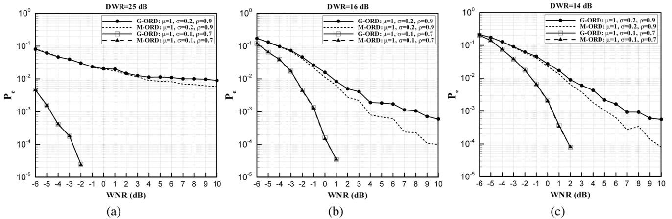
**Fig. 2.** Probability of error of different version of the ORD decoder for two test cases 1)  $\mu = 1, \sigma = 0.2, \rho = 0.9$ , 1)  $\mu = 1, \sigma = 0.1, \rho = 0.7$ . (a) DWR=25 dB, (b) DWR=16 dB, (c) DWR=14 dB
