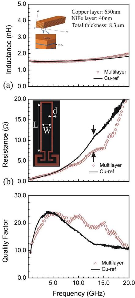
Fig. 1. Comparison of inductance, resistance, and quality factor versus frequency of a single turn *ABMC* inductor (Ind\_33) and its copper counterpart. The insert in (a) shows the sketch of the *ABMC* consisting of 12 periods of bi-layered  $Ni_{80}Fe_{20}$  (40 nm)/ $Cu$  (650 nm) stack on a glass substrate, and in (b) shows the sketch of a single turn inductor.
