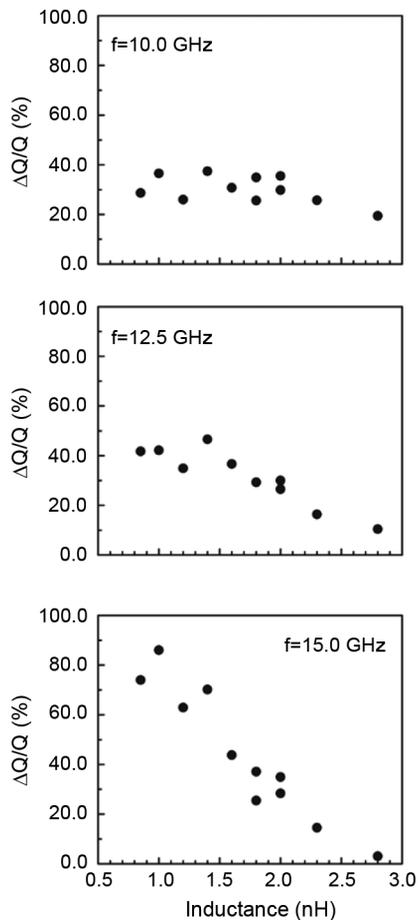
Fig. 2. Comparison of the enhancement of quality factors  $\Delta Q/Q = (Q_{ABMC} - Q_{Cu})/Q_{Cu}$  versus inductance of various inductors (Table 1) at (a) 10.0 GHz, (b) 12.5 GHz, and (c) 15.0 GHz.
