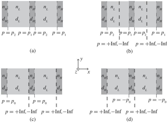
Fig. 2. Representation of pointwise wavenumber of a 1-D Bragg mirror at the interface between higher and lower index layers,  $p_1$  and  $p_2 > p_1$ : (a) the most general case; (b) with one point of singularity within the lower index layer; (c) and (d) with one point of singularity at the interface between higher and lower index layers.
