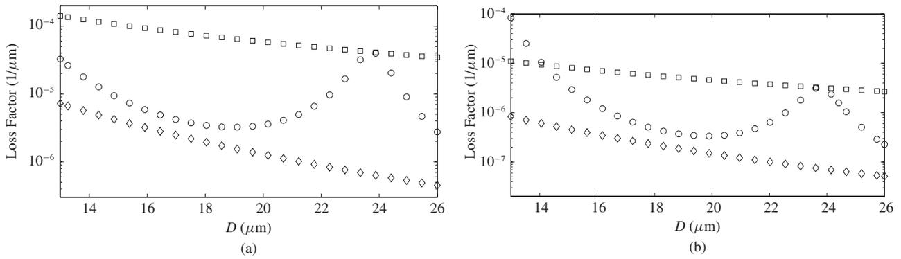
Fig. 6. TE<sub>01</sub> loss factor of the semi-optimum Bragg fiber proposed here (diamond), the quarter-wave Bragg fiber (square), and the modified quarter-wave Bragg fiber (circle) versus core diameter: (a) with two bilayers and (b) with three bilayers in the cladding region.
