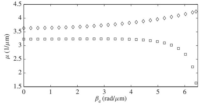
Fig. 4. TE imaginary part of Bloch wavenumber at  $\lambda_0 = 1.55$   $\mu\text{m}$  versus longitudinal propagation constant  $\beta_d$  for the optimum (diamond) and quarter-wave (square) structures having  $n_H = 4.6$  and  $n_L = 1.6$ .
