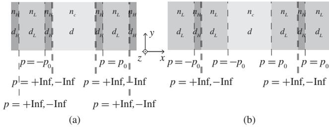
Fig. 5. (a) and (b) Two arrangements to form a planar waveguide sandwiched between optimum 1-D Bragg mirrors with the maximum Bloch confinement.
