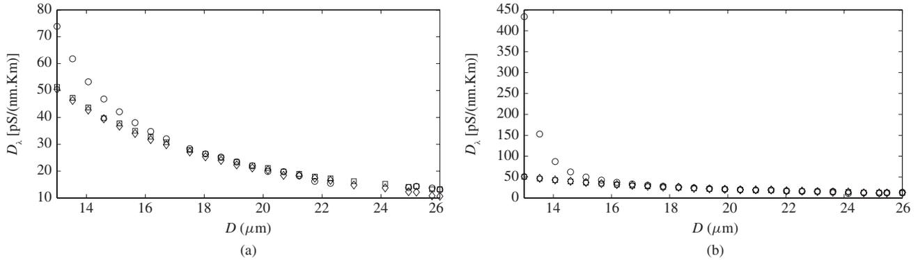
Fig. 7. TE<sub>01</sub> dispersion coefficient of the semi-optimum Bragg fiber (diamond), the quarter-wave Bragg fiber (square), and the modified quarter-wave Bragg fibers (circle) versus the core diameter: (a) with two bilayers and (b) with three bilayers in the cladding region.
