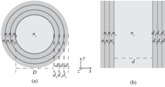
Fig. 1. (a) Bragg fiber with a radially periodic cladding with period  $\Lambda = d_1 + d_2$ , refractive indices and thicknesses are represented by the letters  $n$  and  $d$ , respectively. Note that  $n_c = 1$  for a hollow-core fiber. (b) Corresponding planar structure. It is uniform along the  $y$ -axis.
