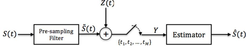
Fig. 1. Sampling-Distortion Model. The signal  $S(t)$  is passed through pre-sampling filter. The output  $\tilde{S}(t)$  is sampled at times  $t_1, t_2, \dots, t_M$ . A noise  $Z$  is added to the signal at the time of sampling. The noisy observations are then used to recover the signal.
