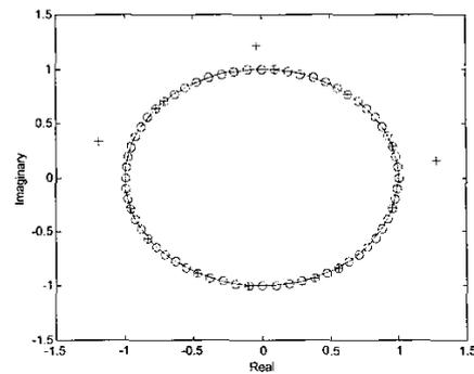
Figure 7: The positions of zeros of the polynomial  $S(z)$  in 8-bit quantization case. The positions of zeros with the form of  $e^{j\frac{2\pi}{N}m}$ , which are on the unit circle, exactly show the location of errors
