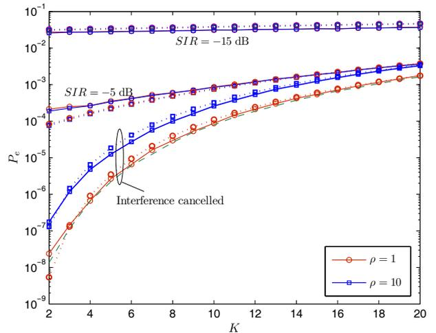
Fig. 6. Multi-user performance of the SE/ST CDMA technique in the presence and after the cancellation of NBI. Solid lines: Monte-Carlo simulation, dotted lines: approximation, dashed line: no interference present.
