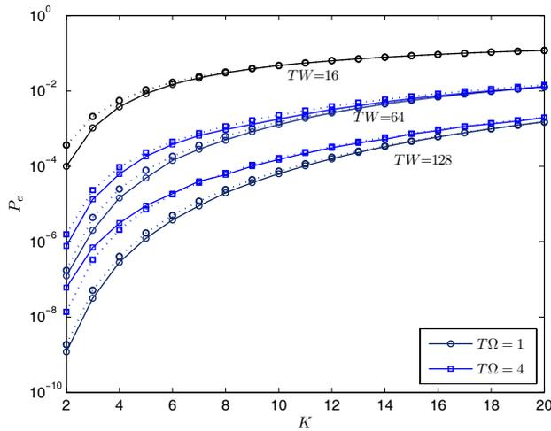
Fig. 4. Performance of the SE/ST CDMA technique versus number of simultaneous users for different time-bandwidth products and spectral code lengths. Solid lines: Monte-Carlo simulation, dotted lines: approximation
