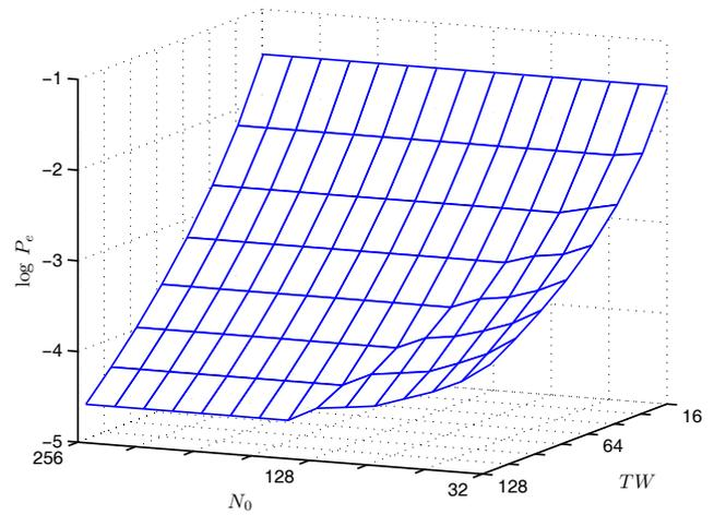
Fig. 5. Performance of the SE/ST CDMA technique versus time-bandwidth product and spectral code lengths for  $K = 8$ , based on the approximation (14).
