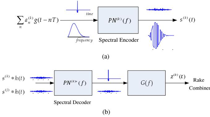
Fig. 1. (a) SE/ST-UWB transmitter, and (b) SE/ST-UWB receiver
