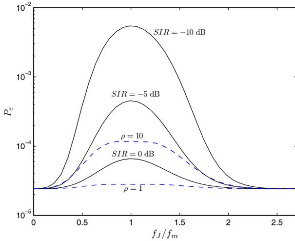
Fig. 7. Performance of the SE/ST CDMA technique in the presence and after the suppression of NBI vs. the jammer's central frequency normalized to  $f_m$ , for different values of jammer's bandwidth and power. Solid lines: before cancellation, dashed lines: after cancellation.
