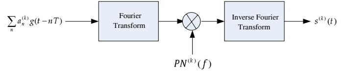
Fig. 2. Spectral encoder implementation using Fourier transformers
