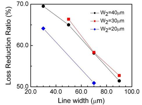
Fig. 6. Comparison of the loss reduction ratio ( $\eta$ ) versus signal line width of ABMC CPWs (Table I), where  $\eta = (\alpha_{\text{Copper}} - \alpha_{\text{ABMC}}) / \alpha_{\text{Copper}}$ .  $\alpha_{\text{Copper}}$  and  $\alpha_{\text{ABMC}}$  are the attenuation constants of the copper and ABMC CPW, respectively.
