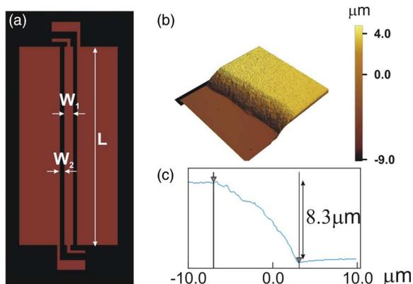
Fig. 1. (a) Sketch of coplanar wave guide. (b) Surface morphology of a CPW measured by atomic force microscopy (AFM). (c) Line scan of CPW by AFM. The thickness of the ABMC layer is around  $8.3 \mu\text{m}$ . Due to the wet chemical etching, the undercut is about  $10 \mu\text{m}$ .
