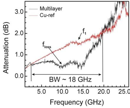
Fig. 4. Comparison of attenuation per centimeter versus frequency of a ABMC CPW (#1) and its copper counterpart.  $f_{\text{loss}}$  is the frequency when the attenuation constant ( $\alpha$ ) of the ABMC CPW reaches minimum. The decrease of  $\alpha$  at frequency  $f_1$  is not clear yet. Since this occurs to both ABMC and copper CPWs, it might be caused by the measurement system.
