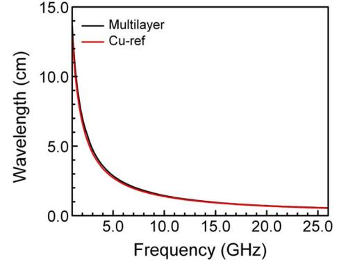
Fig. 5. Comparison of propagation wavelength versus frequency of a ABMC CPW (#1) and its copper counterpart.
