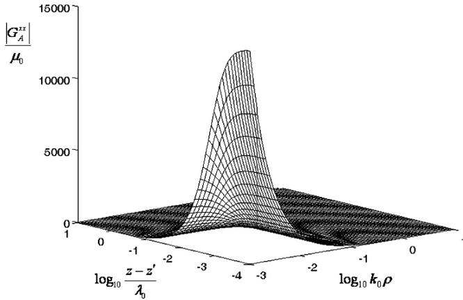
Fig. 4. The amplitude of  $G_A^{xx}/\mu_0$  for the open microstrip structure of Fig. 1 when  $z' = 0$ ,  $h = 0.8\lambda_0$ , and  $\varepsilon_r = 4.3$ .
