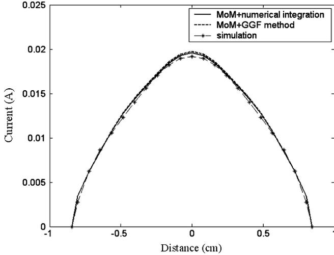
Fig. 6. The current distribution on the horizontal axis of the microstrip antenna of Fig. 3 when  $l = 1.7$  cm,  $w = 0.08$  cm,  $t = 5$  cm,  $\epsilon_r = 4.3$ , and  $f = 4.8$  GHz obtained from the MoM via the GGF method, MoM via the numerical integration and the simulation results.
