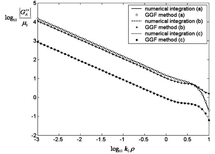
Fig. 8. Comparison of the GGF method with the numerical integration: The amplitude of  $G_A^{xx} \mu_0$  for the open microstrip structure of Fig. 1 when  $z = z' = 0$  and  $f = 4.8$  GHz for: (a)  $h = 5$  cm,  $\epsilon_r = 4.3$ , (b)  $h = 14$  cm,  $\epsilon_r = 4.3$ , and (c)  $h = 14$  cm,  $\epsilon_r = 8.3$ .
