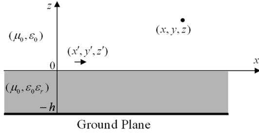
Fig. 1. An infinitesimal horizontal electric dipole above an open microstrip substrate.
