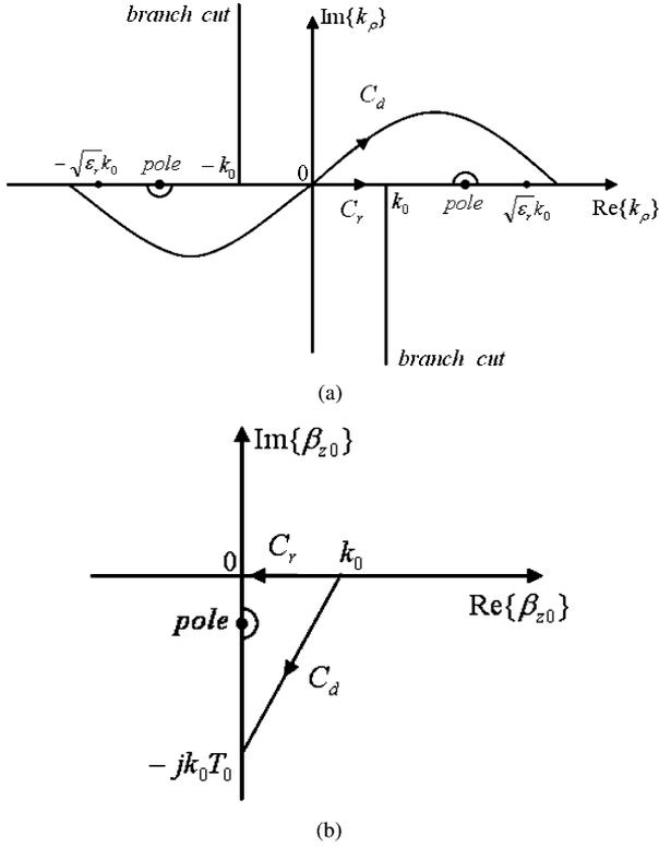
Fig. 2. The integration contours  $C_r$  and  $C_d$ : (a) on the complex  $k_\rho$  plane and (b) on the complex  $\beta_{z0}$  plane.
