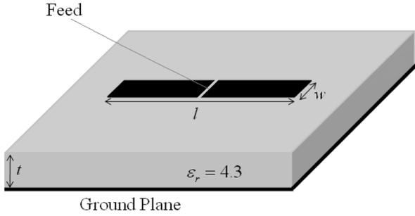
Fig. 3. A planar microstrip antenna on an infinite ground plane.
