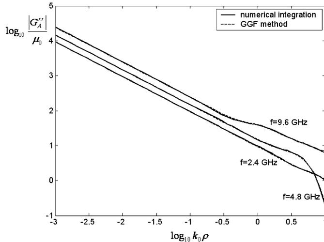
Fig. 7. Comparison of the GGF method with the numerical integration: The amplitude of  $G_A^{xx} \mu_0$  for the open microstrip structure of Fig. 1 when  $z = z' = 0$ ,  $h = 5$  cm, and  $\epsilon_r = 4.3$  at  $f = 2.4$  GHz,  $f = 4.8$  GHz, and  $f = 9.6$  GHz.
