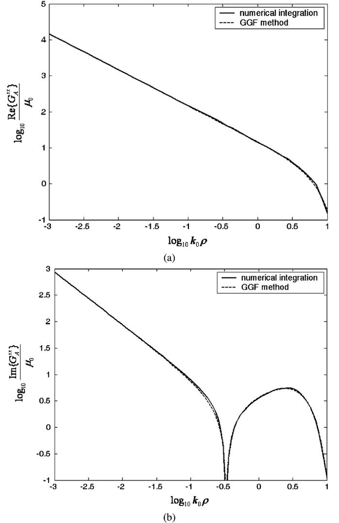
Fig. 5. Comparison of the GGF method with the numerical integration: (a) real and (b) imaginary parts of  $G_A^{xx}/\mu_0$  for the open microstrip structure of Fig. 1 when  $z = z' = 0$ ,  $h = 0.8\lambda_0$ , and  $\varepsilon_r = 4.3$ .
