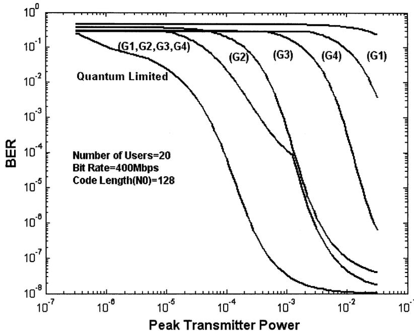
Fig. 6. BER versus peak transmitter power for quantum-limited case, and a typical system with one amplifier or four amplifiers.
