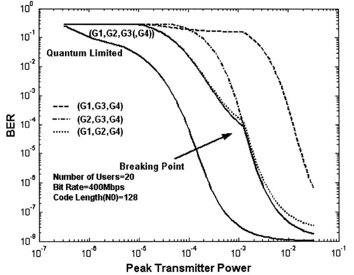
Fig. 11. BER versus peak transmitter power for quantum-limited case, and a typical system with three and four amplifiers. The breaking point in the above curve is due to the saturation effect of  $G_1$  beyond which the gain of the first amplifier  $G_1$  is set to unity, i.e., 0-dB gain.
