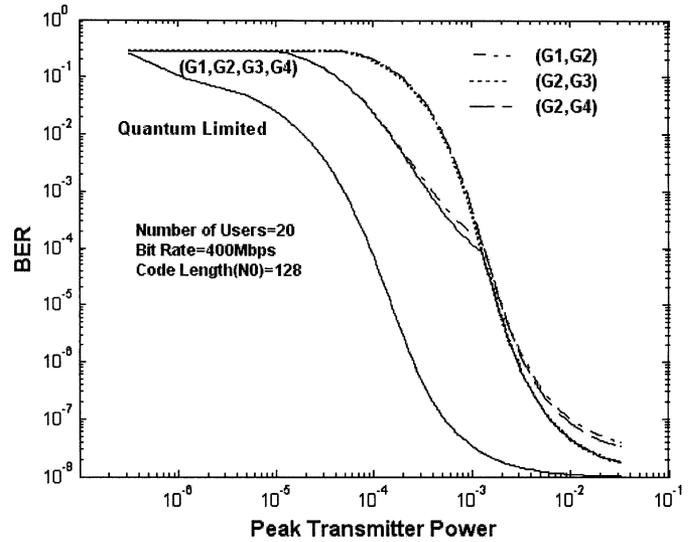
Fig. 8. BER versus peak transmitter power for quantum-limited case, and a typical system with two and four amplifiers.
