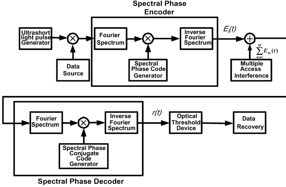
Fig. 1. Typical block diagram of a lossless CULP-CDMA system.
