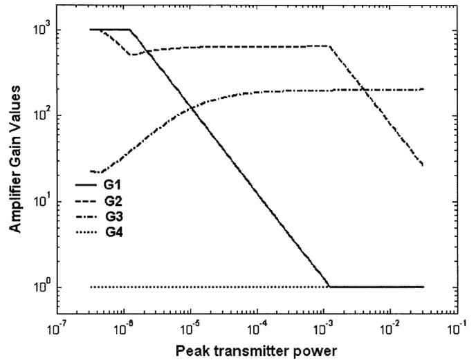
Fig. 12. Amplifier gain values versus peak transmitter power for four amplifier system, i.e.,  $(G_1, G_2, G_3, G_4)$ .
