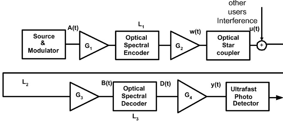
Fig. 3. System model representation for CULP-CDMA system with multiple optical amplifiers.
