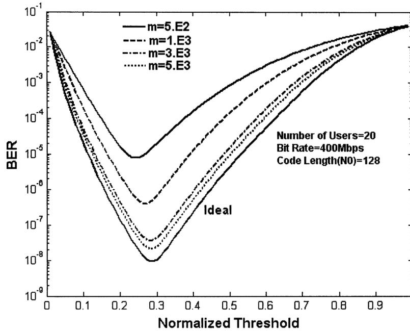
Fig. 4. BER versus normalized threshold for ideal and quantum-limited cases.
