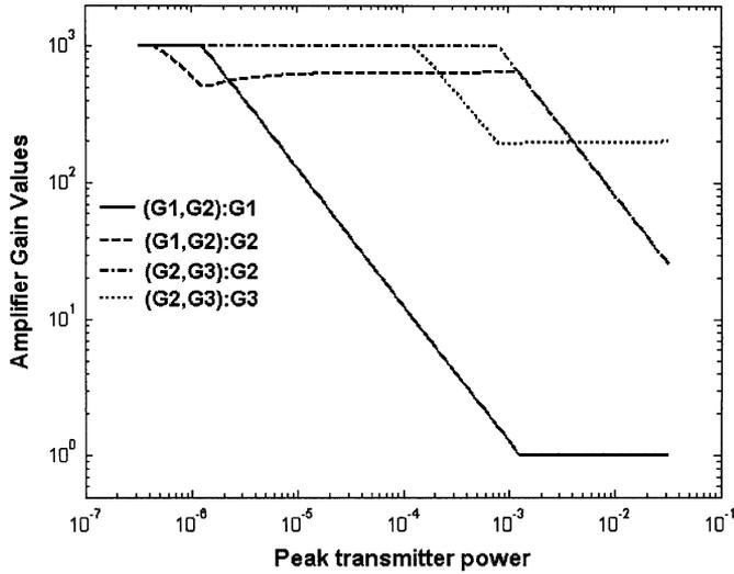
Fig. 10. Amplifier gain values versus peak transmitter power for two types of two-amplifier systems.
