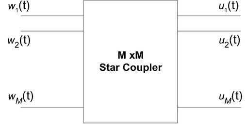
Fig. 2. Typical  $M \times M$  star coupler:  $u_i(t) = (1/\sqrt{M}) \sum_{k=1}^M e^{j\phi_{ik}} w_k(t)$ .
