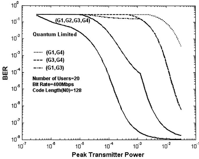
Fig. 9. BER versus peak transmitter power for quantum-limited case, and a typical system with two and four amplifiers.
