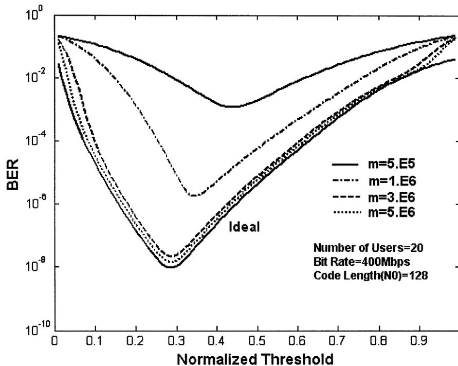
Fig. 5. BER versus normalized threshold for ideal case and a typical system without amplifiers.
